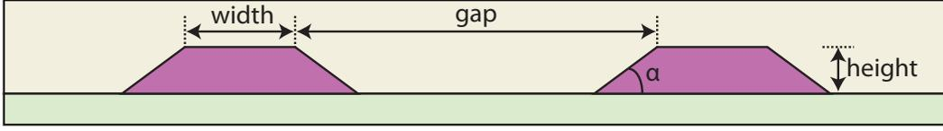
**Figure 4.4:** Coupler geometry as generated by FieldDesigner. Based on this geometry, the effective propagation modal indices are calculated from the entered refractive indices of the different materials and waveguide dimensions.
