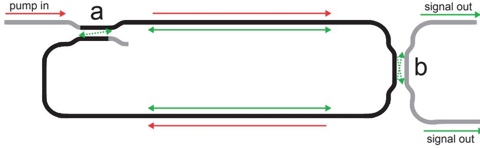
**Figure 6.3:** Diagram of an integrated Nd-doped channel waveguide laser with a loop cavity. Pump power is coupled in the upper waveguide and will traverse coupler (a) without coupling. Laser light is generated in the cavity, (colored black) and is partially coupled out by coupler (b). Since laser light travels in the loop both clockwise and anti-clockwise, laser light is coupled into the upper channel on the right and the lower channel on the right.
