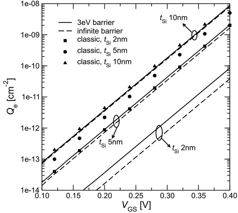
Figure 2.2: QM and classical inversion charge density for  $t_{\text{Si}}$  2, 5 and 10 nm.
