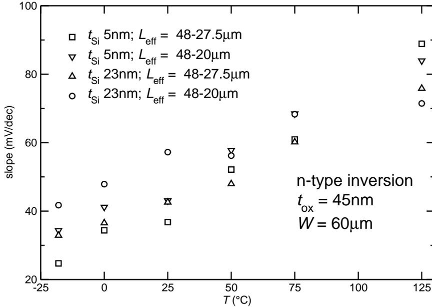
Figure 3.21: Subthreshold slope vs the temperature (*n*-type inversion). Extracted using  $C_{\text{min}} = 2.3 \text{ nF}/\mu\text{m}^2$  and  $C_{\text{max}} = 5.5 \text{ nF}/\mu\text{m}^2$ .
