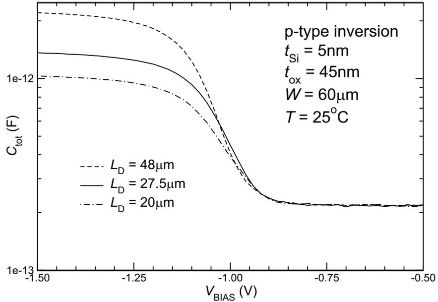
Figure 3.13: Single  $CV$  measurement (hole inversion) on PiN diodes with  $L_D$  20, 27.5 and 48  $\mu\text{m}$ .
