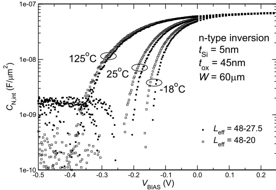
Figure 3.18: Differential  $CV$  measurement ( $n$ -type inversion) for  $T = -18, 25, 125$  ( $^{\circ}\text{C}$ ).
