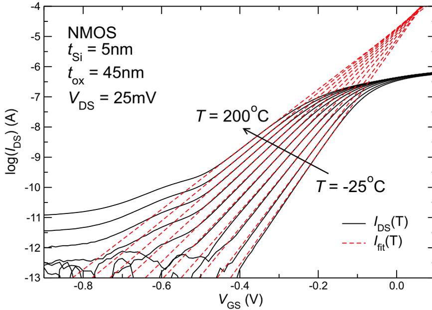
Figure 3.5: Temperature dependent  $I_{DS}(V_{GS})$  measurements on the thinnest NMOS device.
