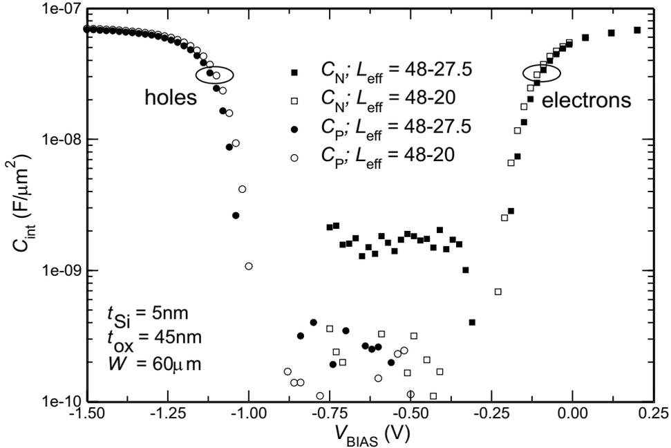
Figure 3.17: Differential *CV* measurement, showing the electron and hole inversion at room temperature.  $L_{\text{eff}}$  is given in ( $\mu\text{m}$ ).
