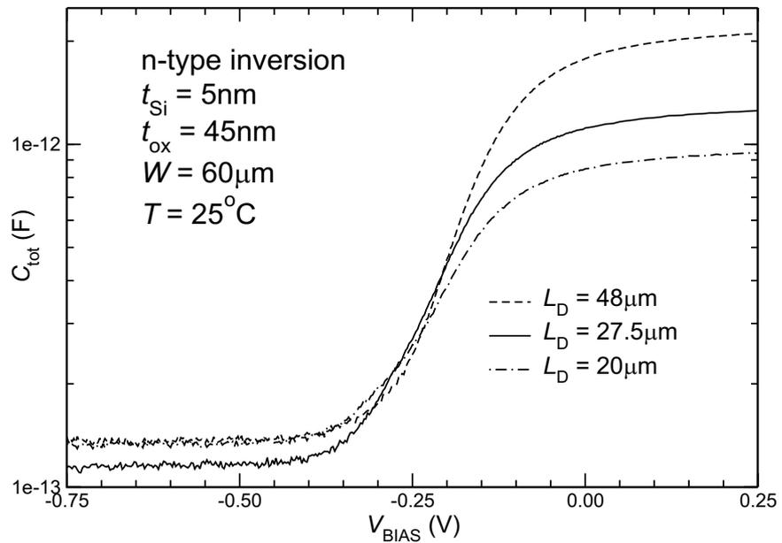
Figure 3.14: Single  $CV$  measurement (electron inversion) on PiN diodes with  $L_D$  20, 27.5 and 48  $\mu\text{m}$ .
