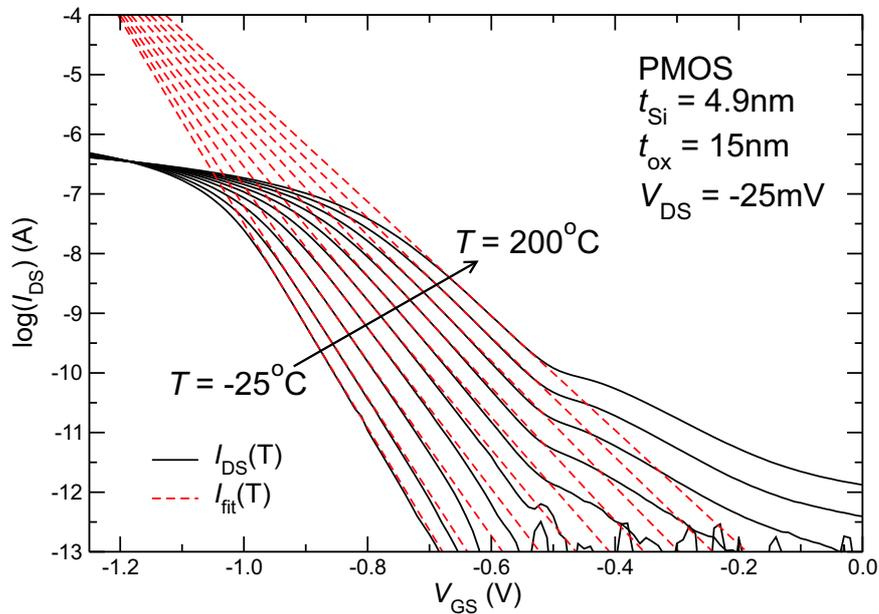
Figure 3.4: PMOS  $I_{\text{DS}}(V_{\text{GS}})$  for  $T = -25 \dots 200^{\circ}\text{C}$  (solid lines); the dashed lines have been fit to the ideal subthreshold region to eliminate the influence of channel resistance on the band gap extraction.
