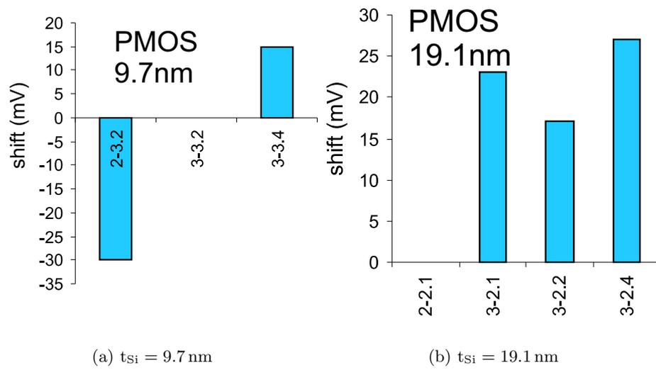
Figure A.2: Shift in  $V_{GS}$  across all PMOS devices on 3 wafers
