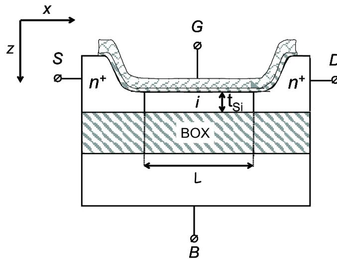
Figure 3.1: Schematic cross-section SOI DG NMOS
