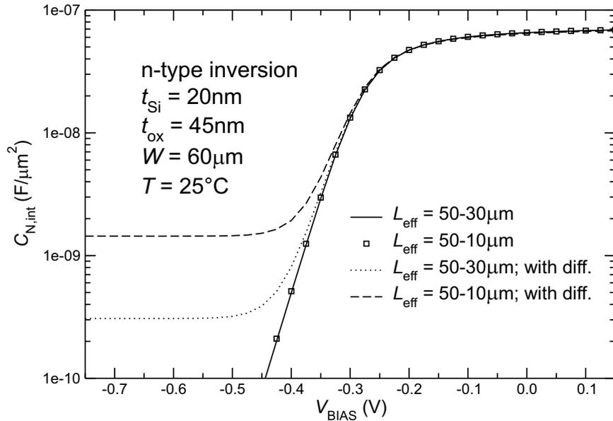
Figure 3.20: Simulated  $CV$  characteristic ( $n$ -type inversion) with and without ‘diffusive’ junctions, clearly showing that the diffused dopants strongly affect the depletion capacitance. The difference between long devices should be observed to reduce the influence of the diffusive junctions.
