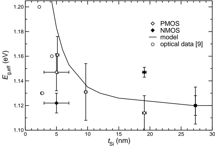
Figure 3.11: Change in effective band gap, extracted from the slope of  $I_{rat}$ .
