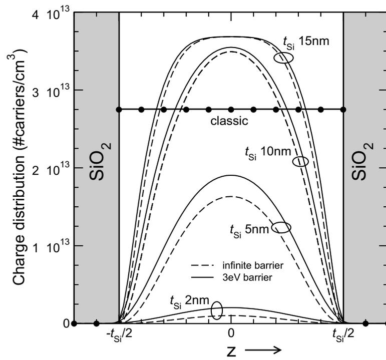
Figure 2.1: QM and classical charge distribution throughout the channel depth for several  $t_{\text{Si}}$ ; Calculated with  $N_{\text{C}} = 2.8 \times 10^{19} \text{ cm}^{-3}$ ,  $N_{\text{V}} = 1.04 \times 10^{19} \text{ cm}^{-3}$ ,  $T = 300 \text{ K}$  and  $V_{\text{GS}} = 0.2 \text{ V}$ .
