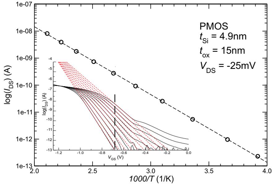
Figure 3.9:  $I_{\text{DS}}(T)$  at  $V_{\text{GS}} = -0.7$  V (see inset) for DG PMOS with  $t_{\text{Si}} = 4.9$  nm. All data points are almost perfectly on the exponential regression line (dashed line), except for the two outermost points, which show a small deviation.
