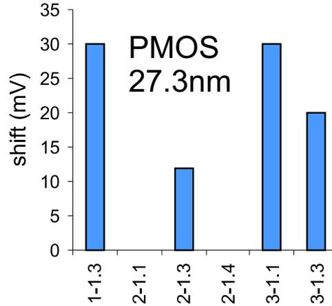
Figure 3.8: Shift in  $V_{GS}$  for the thickest PMOS device, for which  $t_{Si} = 27.3$  nm on wafer 2.
