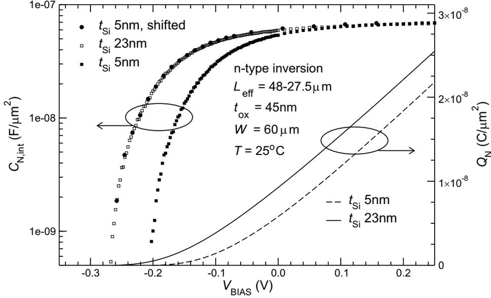
Figure 3.19: Differential  $n$ -type capacitance and inversion charge for  $t_{\text{Si}}$  equal to 5 nm and 23 nm. The solid circles denote the shifted characteristic of the 5 nm device.
