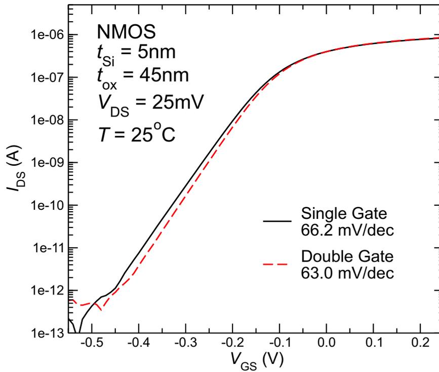
Figure 3.3: typical  $I_{DS}$  curve for SG and DG operation mode.
