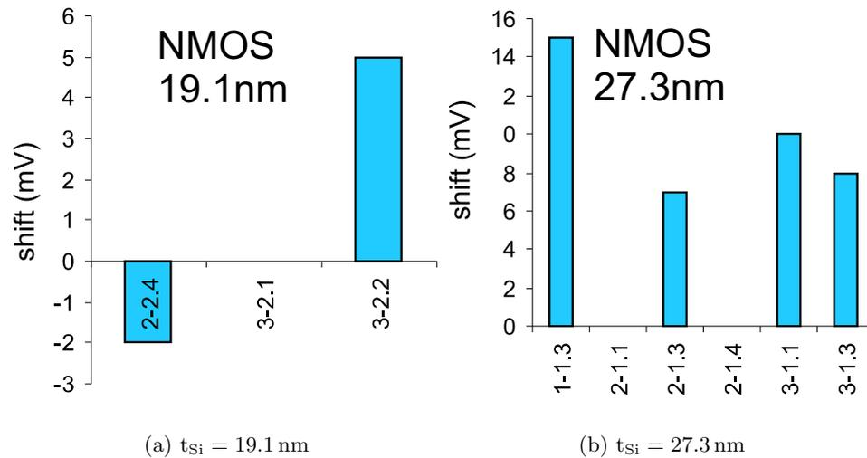
Figure A.1: Shift in  $V_{GS}$  across all NMOS devices on 3 wafers
