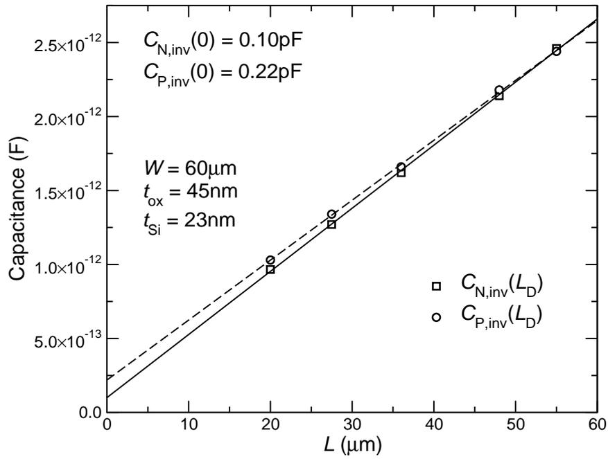
Figure 3.15: The hole ( $C_{P,inv}$ ) and electron ( $C_{N,inv}$ ) capacitance in strong inversion vs  $L_{\text{ch}}$ , demonstrating a clearly linear relation between  $C_{\text{inv}}$  and  $L_{\text{ch}}$ . The parasitic capacitances ( $C_{P,\text{par}}$  and  $C_{N,\text{par}}$  for holes and electron resp.) can be obtained by extrapolating the curves to  $L_{\text{ch}} = 0 \mu\text{m}$ , giving  $C_{P,\text{par}} = 0.22 \text{ pF}$  and  $C_{N,\text{par}} = 0.10 \text{ pF}$ .
