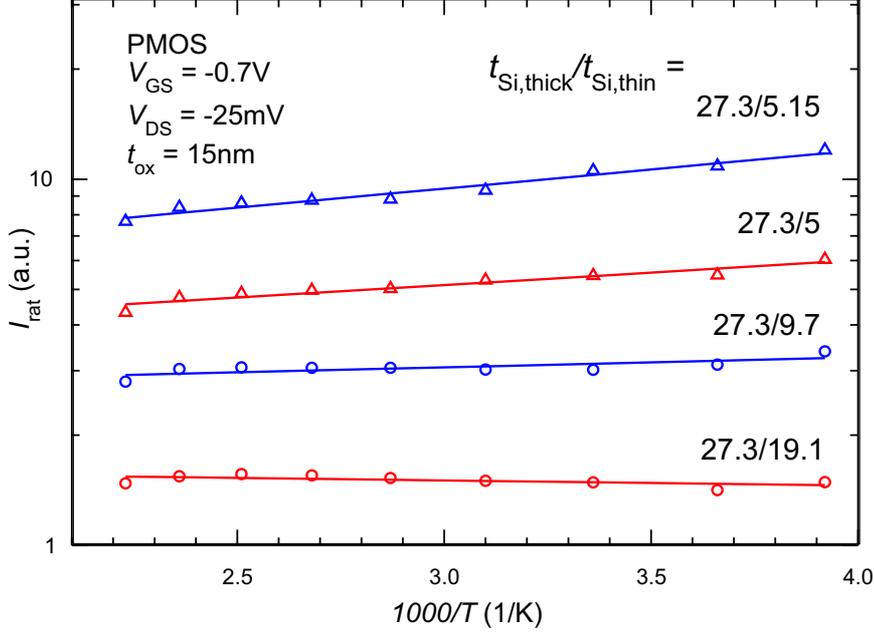
Figure 3.10:  $I_{\text{thick}}/I_{\text{thin}}$  ( $= I_{\text{rat}}$ ) vs temperature, for the DG PMOS devices with the 27.3 nm device as reference. Note that  $I_{\text{rat}}$  increases for thinner layers, which is either due to a lower mobility or a reduced DoS. The layer thickness of the 5 nm device is given with  $\pm 2$  nm accuracy, and  $t_{\text{ox}}$  of this device is 45 nm.
