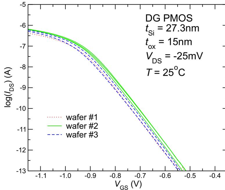
Figure 3.7: Shift along  $V_{GS}$ , obtained from the thickest DG PMOS device on different wafers. The layer thickness is determined accurately only for devices on wafer 2, on which the thickest device is 27.3 nm. Detailed information on device parameters and wafer numbers can be found in appendix B.
