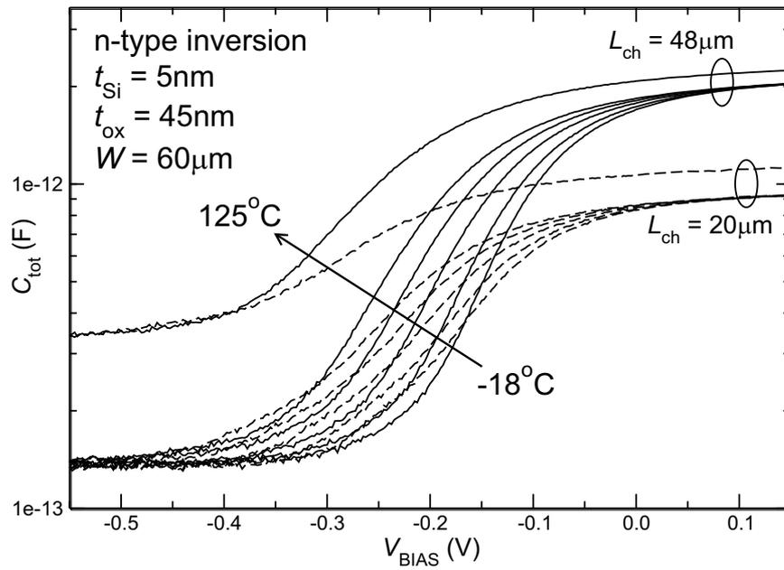
Figure 3.16: Single  $CV$  measurement ( $n$ -type inversion) at  $T = -18, 0, 25, 50, 75, 125$  ( $^{\circ}\text{C}$ ), demonstrating the different temperature dependence of the implanted regions (dominant in depletion region) and the intrinsic channel region (dominant in strong inversion).
