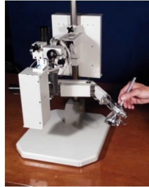
Figure 2.2: Haptic device: Freedom6S
