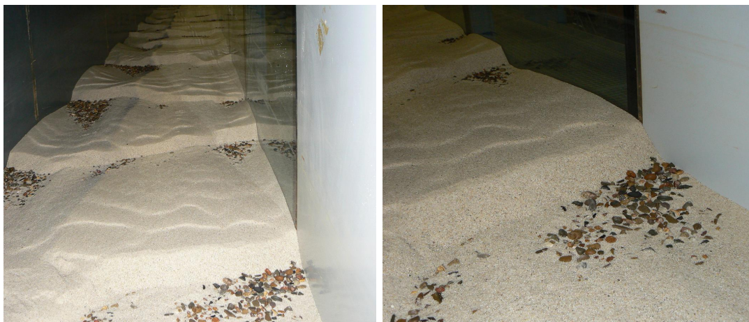
Figure 1.1: Example of partial transport, showing supply limited bed forms and gravel patches of a pavement layer
