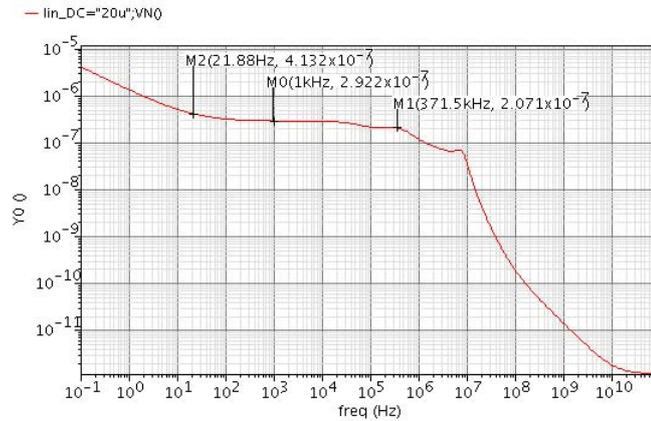
Figure 4.10: Spectral noise density plot - Output noise voltage
