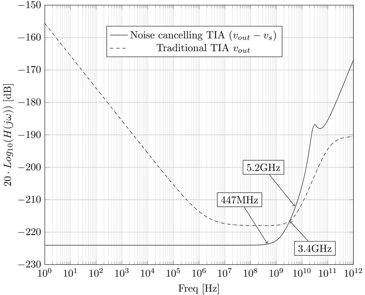
Figure 5.4: Frequency response of the input referred noise
