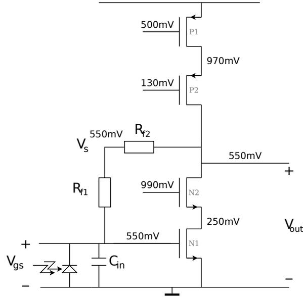
Figure A.1: Bias conditions of the single stage cascoded TIA with resistive feedback
