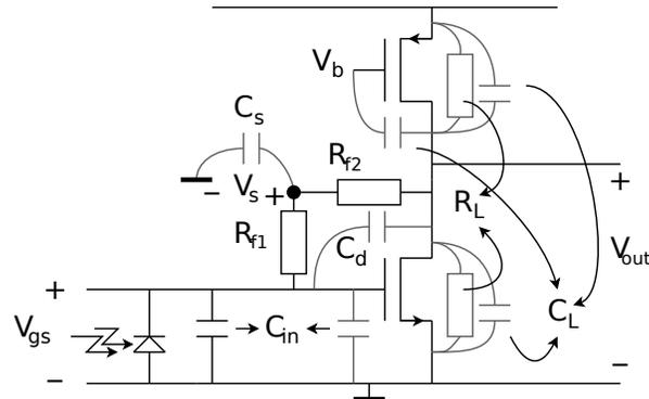
Figure 4.4: Single stage TIA with its parasitics
