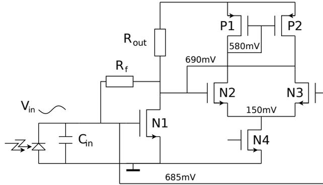
Figure 4.16: Bias conditions of the bandwidth extension TIA
