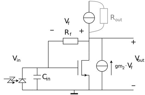
Figure 4.9: Common source TIA with steered current source
