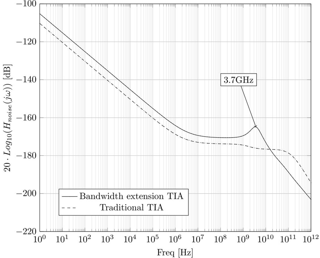
Figure 5.6: Output noise density of the traditional TIA and the bandwidth extension TIA
