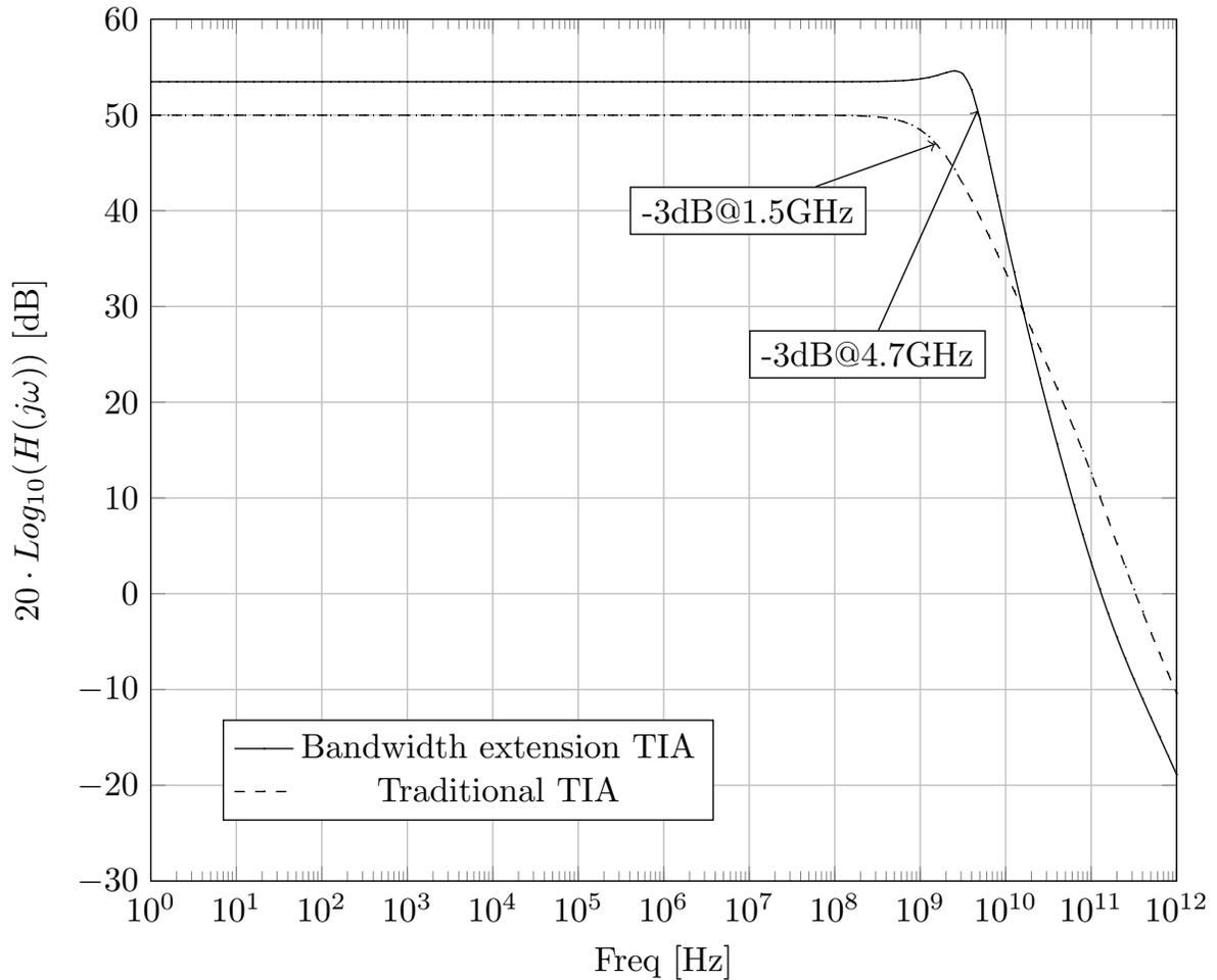
Figure 5.5: Frequency response of the traditional TIA and bandwidth extension TIA
