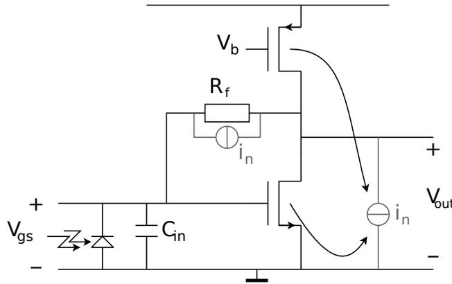
Figure 3.3: Noise sources of the common source TIA
