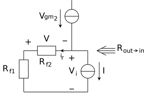
Figure 4.8: Effect of the asymmetric resistance on two resistors
