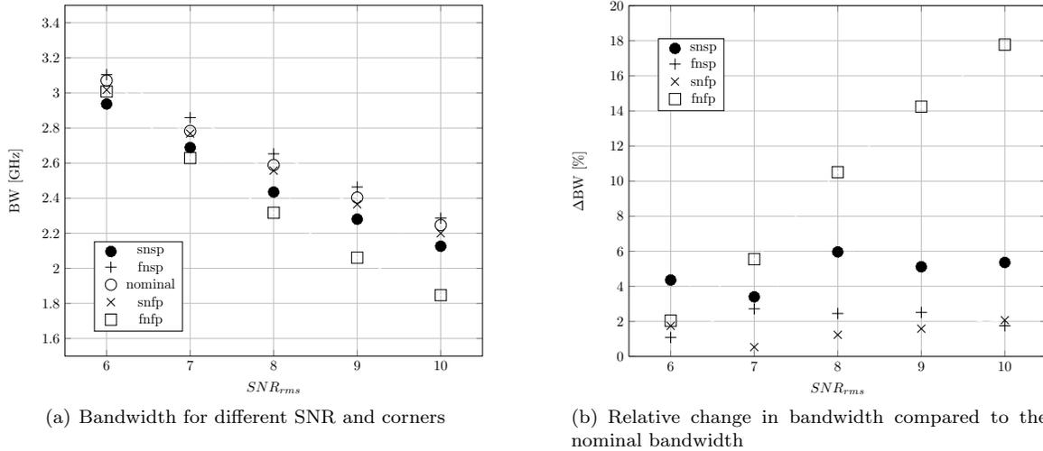
Figure 5.7: Spread simulation for different corners swept over SNR
