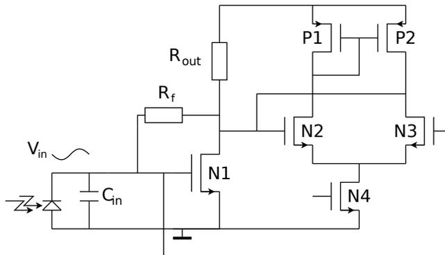
Figure 4.13: Transistor implementation of the common source TIA with bandwidth extension
