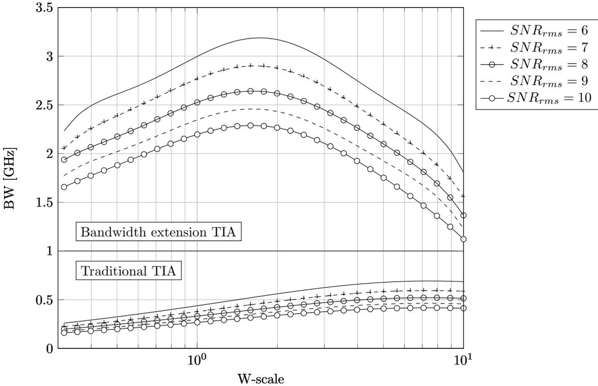
Figure 5.8: Bandwidth for the traditional and bandwidth extension TIA, for constant SNR ( $L_T = 60nm$ )
