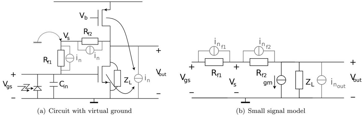
Figure 4.2: Common source TIA with its noise sources
