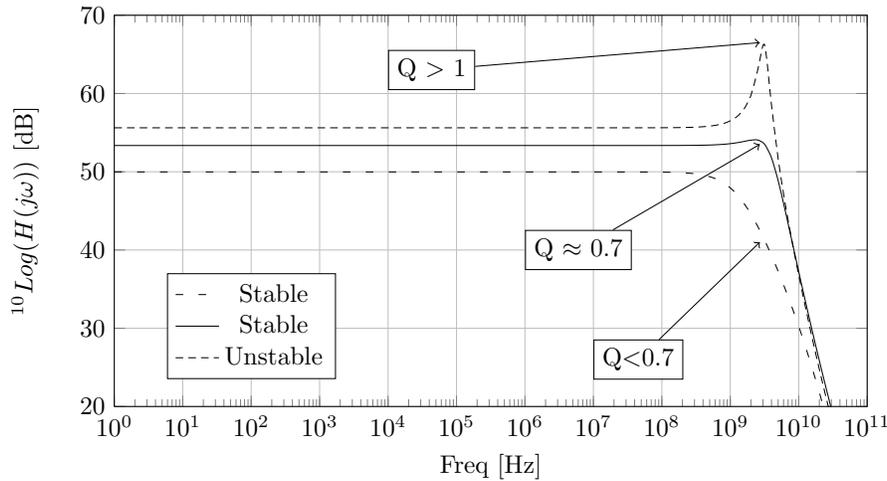
Figure 4.11: Frequency transfer for different Q factors
