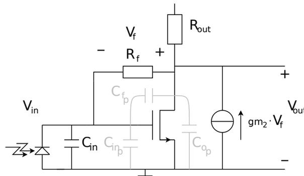
Figure 4.10: Parasitic capacitances of the common source TIA with bandwidth extension
