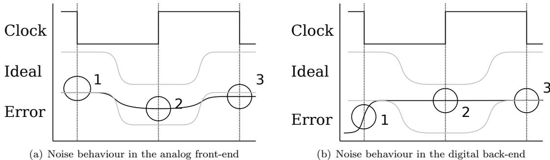
Figure 2.1: Overview of the bit error mechanisms
