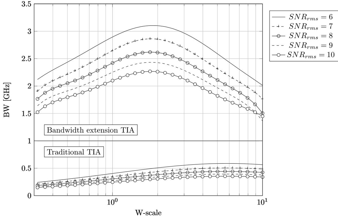
Figure 5.9: Bandwidth for the traditional and bandwidth extension TIA, for constant SNR ( $L_T = 100\text{nm}$ )
