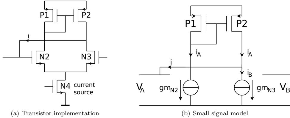
Figure 4.12: Voltage controlled current source
