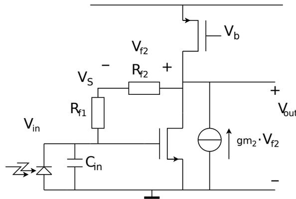
Figure 4.7: Asymmetric resistance in the common source TIA
