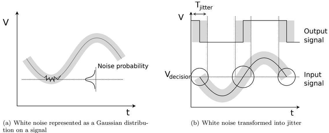
Figure 2.3: Noise and jitter representations
