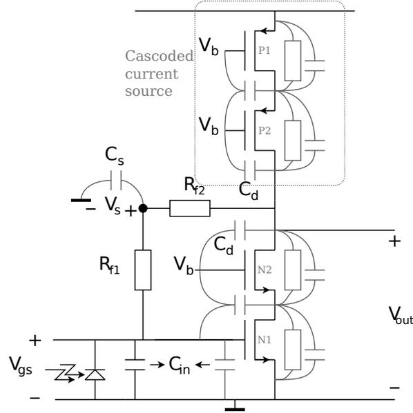
Figure 4.5: Single stage cascoded TIA with its parasitics
