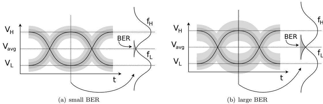
Figure 2.2: Eyediagram with gaussian amplitude noise on  $V_L$  and  $V_H$
