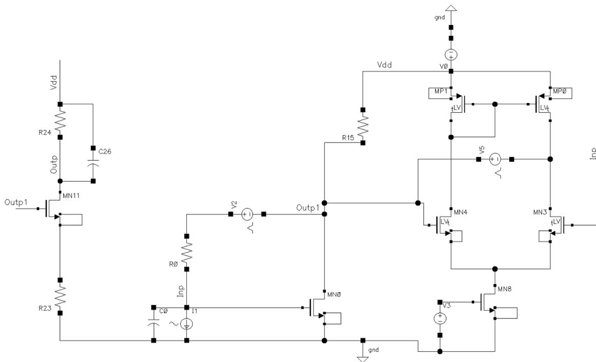
Figure B.1: Cadence circuit of the bandwidth extension TIA
