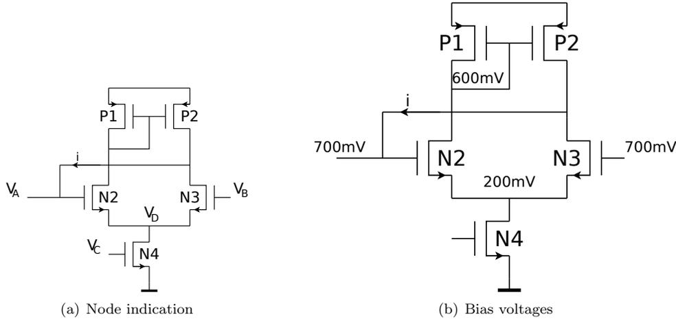
Figure 4.15: Voltage controlled current source
