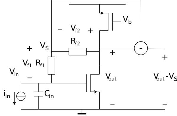
Figure 4.3: Noise cancelling TIA with schematic subtraction node
