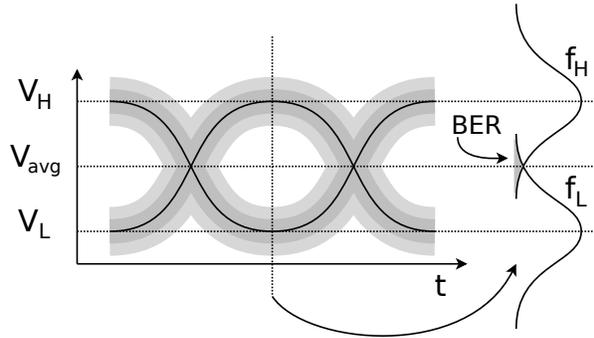
Figure 2.5: Overview of the bit error probability in the analog domain
