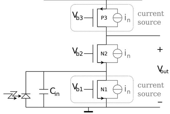
Figure 3.1: Common gate TIA with its noise sources
