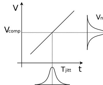
Figure 2.4: Transformation of voltage noise to timing jitter at a threshold [10]
