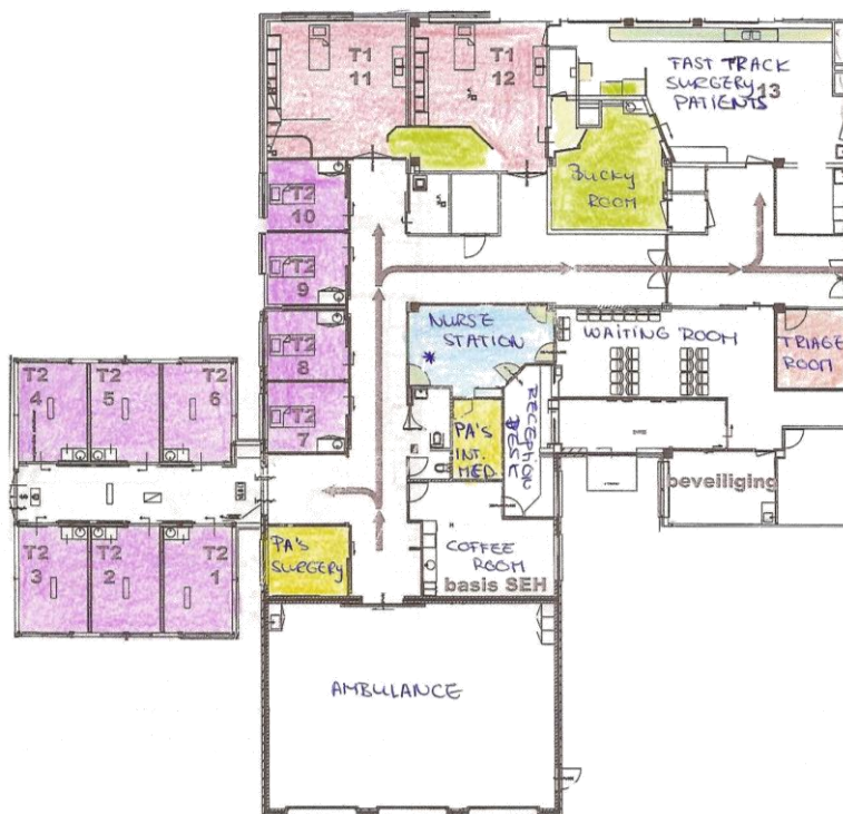
Figure 25: Floor-plan of the emergency department. Purple = general patient room, red = trauma room, green = x-ray facilities, blue = nurse workstation, yellow = residents workstation, orange = triage room.
