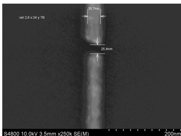
Figure 6.2: SEM results of line with gap structure from Delft
