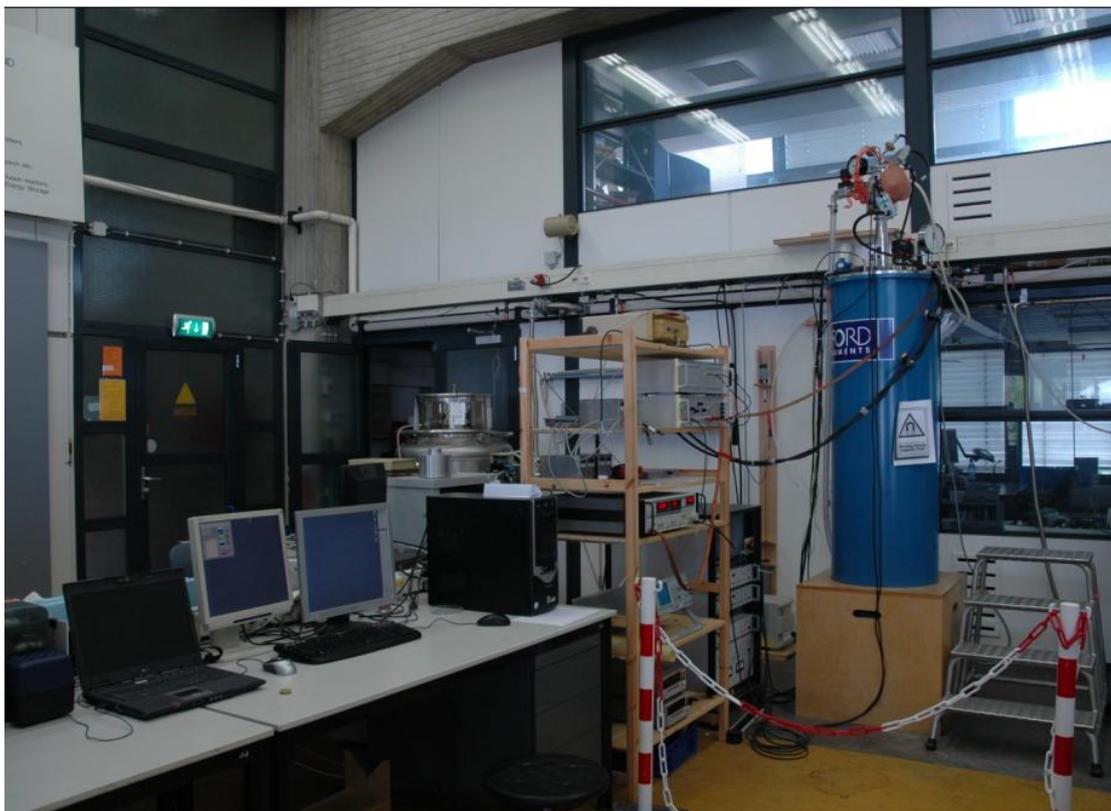
It is essential to use a cryogenic setup to observe the Aharonov-Bohm effect. The system consists of some major parts named as – Heliox VL cryostat, Superconducting magnet, measurement electronics and control software. In this chapter, mainly measurement electronics will be discussed.
