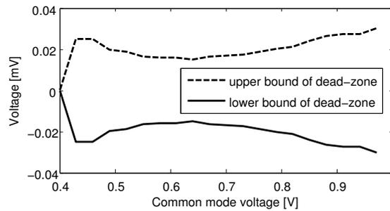
Figure 5.11: Dead-zone: range in which the comparator output is not between 0.2 and 0.8 of supply voltage of 1V.
