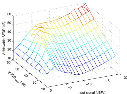
Figure 3.11: Achievable SFDR for Gaussian distributed dither and signal attenuation. MATLAB code snippet can be found in Appendix C.2.
