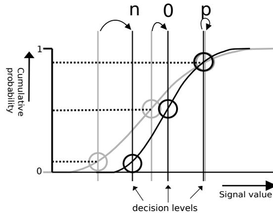
Figure 4.2: Reference levels are adapted to CDF changes: a positive offset is introduced and the amplitude is decreased.
