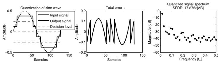
Figure 3.6: 2-bit Quantization of a sine wave and the quantization error.
