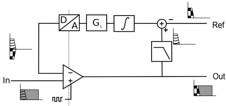
Figure 4.6: Decision level loop effect in frequency domain. The low-frequency content of the input signal is filtered out and the reference signal is added. The reference signal sets the decision level. The small spectra illustrate how frequency content is subtracted and added.
