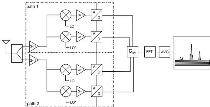
Figure 2.9: Quadrature mixing XF cross-correlation spectrum analyzer ( $LO^*$  denotes the 90 degrees shifted oscillator signal phase)
