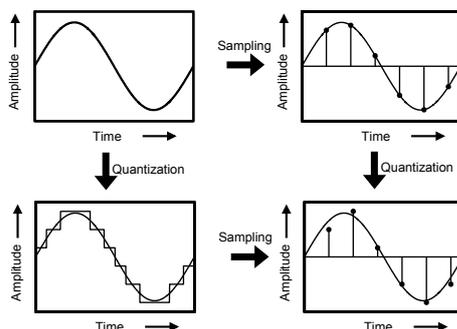
Figure 3.1: Analog to digital conversion: Sampling and Quantization
