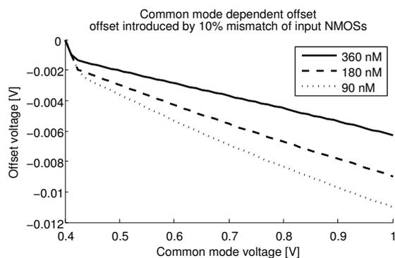
Figure 5.6: Illustration of common mode dependent offset. The offset is introduced by increasing the length of M5 by 10%. In the plot the three lines correspond to the three lengths of the input phase tail NMOS (M9).
