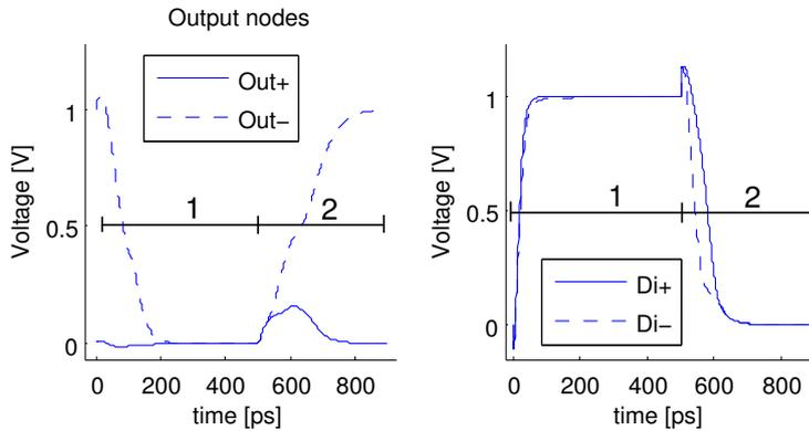
Figure 5.3: Internal and output nodes of comparator for a voltage difference of 150 mV. 1) reset phase. 2) compare phase
