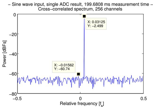
Figure 4.21: Total IF front-end simulation, spectrum (when settled), settings used shown in Table 4.2
