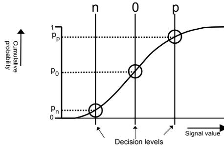
Figure 1.3: CDF-based AGC ADC principle: decision levels depend on system settings and input CDF
