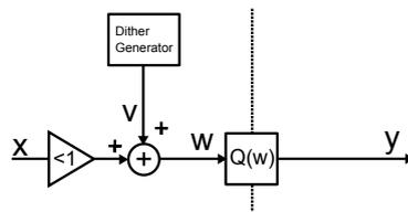
Figure 3.10: Dithered quantizer with attenuated input signal.
