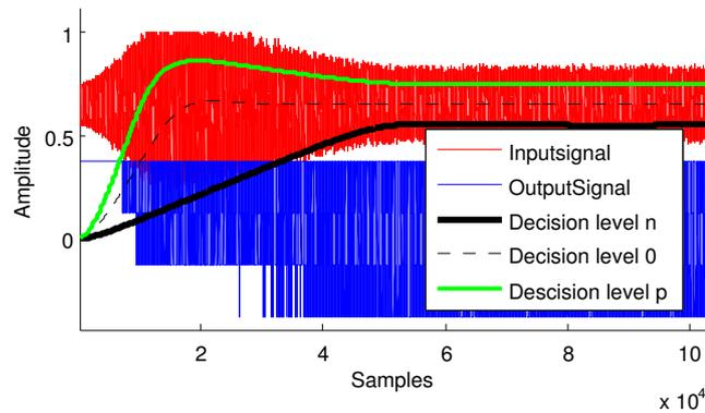
Figure 4.23: Clipping of input signal while settling. 4.3
