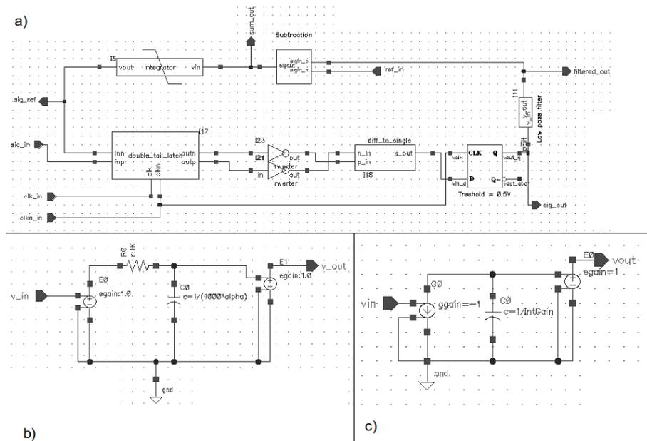
Figure 5.12: a) Single decision level loop. b) Ideal low pass filter. c) Ideal analog integrator
