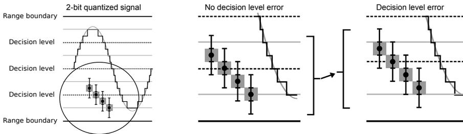
Figure 3.26: Decision level error effect on input signal ranges (gray areas), which lead to an output value
