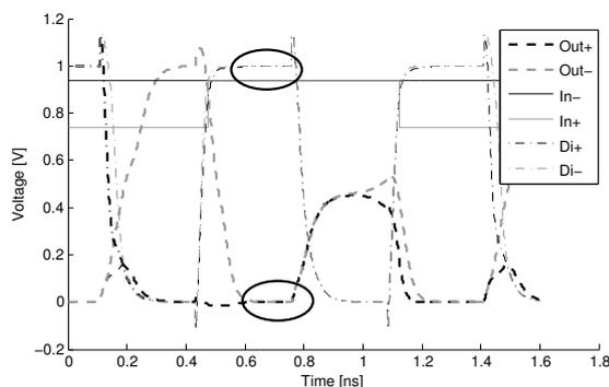
Figure 5.10: Static hysteresis is obscured by noise and not degrading the performance below toleration. The  $Di$  and output nodes are reset properly as indicated by the ellipses. The voltage difference is  $< 1\mu V$  at the end of the reset stage.
