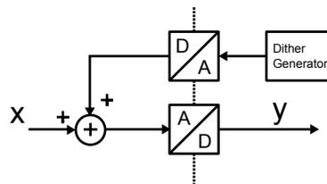
Figure 3.19: Digitally dithered quantizer
