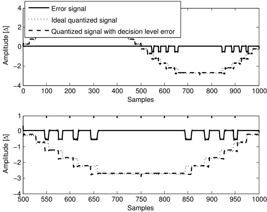
Figure 3.27: Time domain representation of decision level variation. Obtained by calculating the frequency components of  $e_{EQ_e}$ , when  $D = 2$  and  $\alpha = 0.8$ . MATLAB code in Appendix C.4
