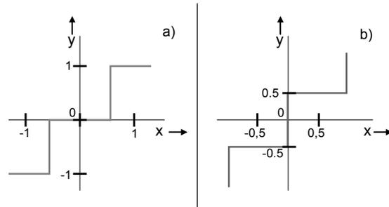
Figure 3.3: a) Midtread quantizer transfer function. b) Midrise quantizer transfer function.
