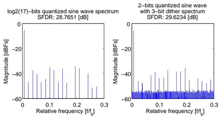
Figure B.3: Spectra of a  $\log_2(17)$ -bits equivalent quantizer and the 3-bit triangular dithered 2-bit quantizer: they have approximately the same SFDR. (MATLAB code in appendix C.3)
