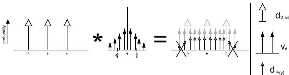
Figure B.2: Convolution of triangular dither PDF and quantizer decision levels result in decision level distribution.
