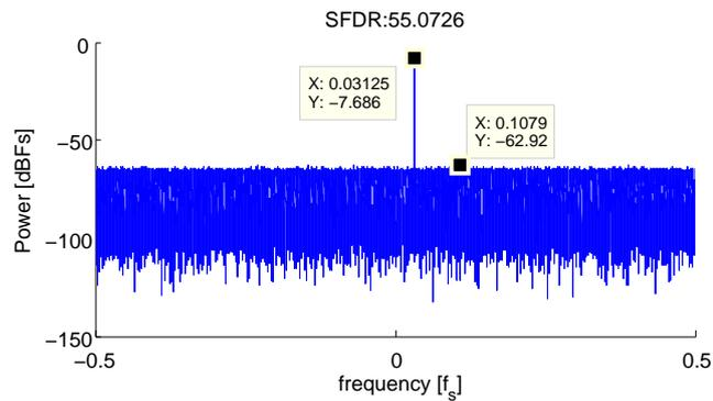
Figure 4.26: Spectrum when ADC is settled, The fundamental tone now has a amplitude of -7.7 dBFS. Settings used shown in Table 4.4
