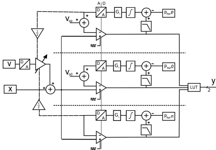
Figure 4.29: Total ADC with offsets added to upper and middle comparator.
