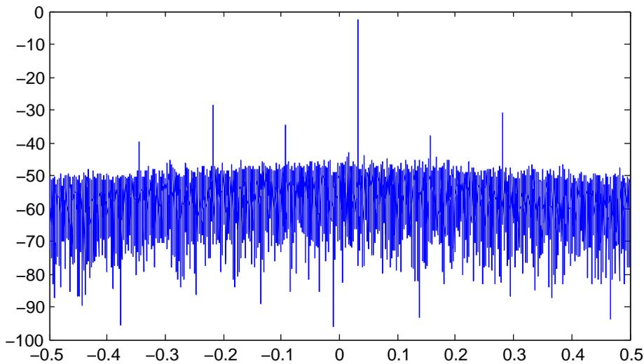
Figure 5.13: Spectrum when no track and hold is used.
