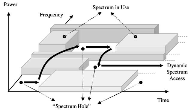
Figure 1.1: A cognitive device jumps from spectrum hole to spectrum hole [1].
