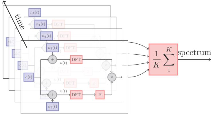
Figure 2.3: Block diagram of the operation of a cross-correlation spectrum averaging front-end. [4]
