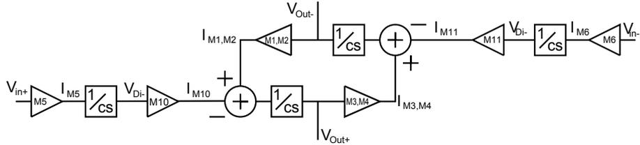
Figure 5.4: Block diagram representation of comparator
