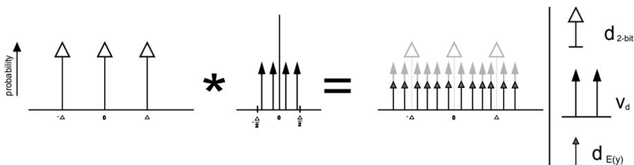
Figure 3.22: Convolution of rectangular dither PDF and quantizer decision levels result in decision level distribution.
