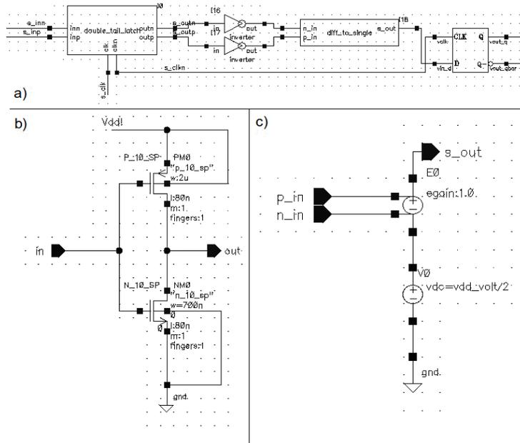
Figure 5.7: a) Simulation of the comparator. b) Inverter to take into account capacitive load. c) Ideal differential to single ended conversion.
