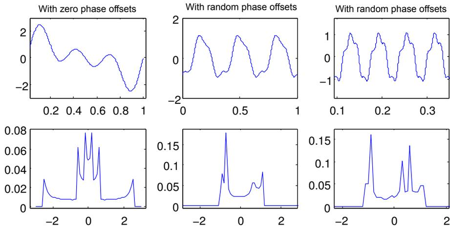
Figure 4.17: Sums of multiple sine waves with different frequency and phase offset result in symmetrical or asymmetrical PDFs. The three signals are the sum of three sinusoids only with different phase differences.
