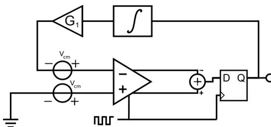
Figure 5.8: Test-bench for investigating offset
