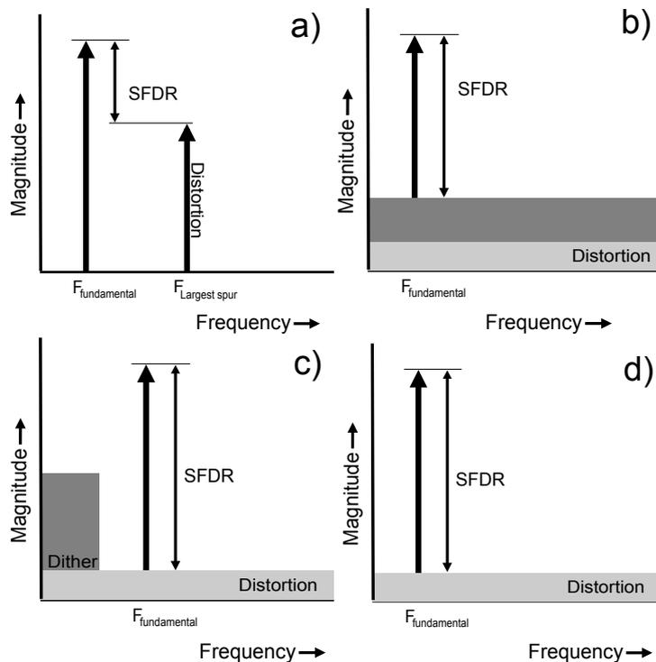
Figure 3.12: Dithering schemes and effect on SFDR: a) no dither. b) non-subtractive dither. c) band-limited dither. d) subtractive dither.
