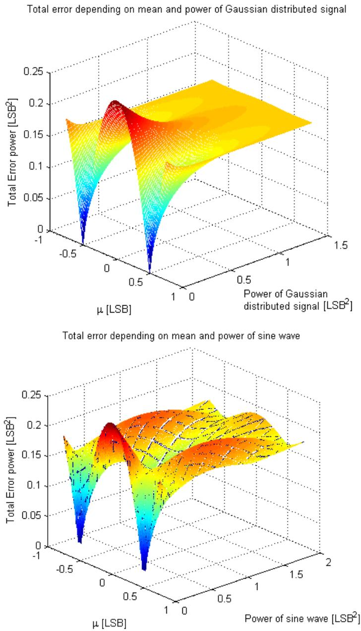
Figure 3.16: Total error depending on mean ( $\mu$ ) and power of Gaussian distributed signal (top) and sine wave (bottom) when dithered with a rectangular dither signal.
