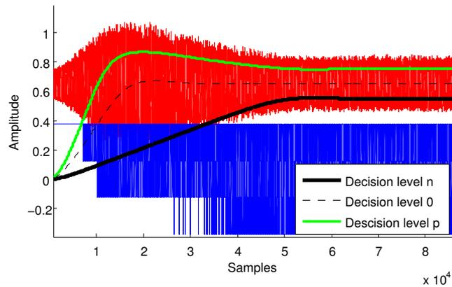
Figure 4.22: Settling of the ADC, settings used shown in Table 4.3
