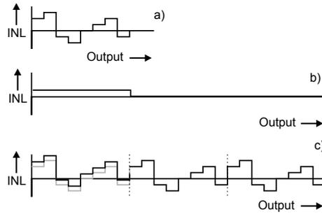
Figure 3.25: Repetitive INL due to INL of dither DAC. a) INL of the dither DAC. b) INL of the 2-bit quantizer. c) Statistical INL of the dithered quantizer.
