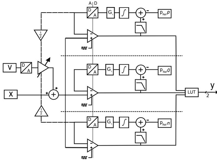
Figure 4.10: Total ADC with scaled dither added to the input signal
