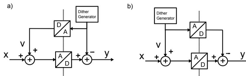
Figure 3.9: Subtractive dither quantizer. The dither source can be in: a) digital or b) analog domain.
