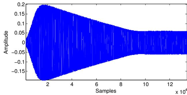
Figure 4.25: Scaled dither signal, settings used shown in Table 4.4
