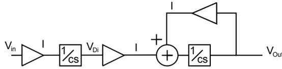
Figure 5.5: Block diagram representation of comparator, assuming perfect symmetry between parallel branches.
