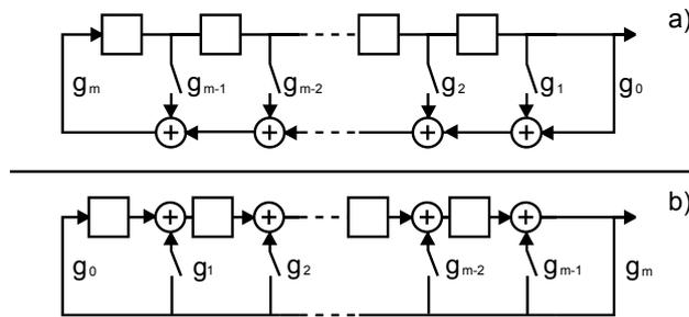
Figure 3.29: Linear shift feedback registers. a) the Fibonacci generator. b) the Galois generator
