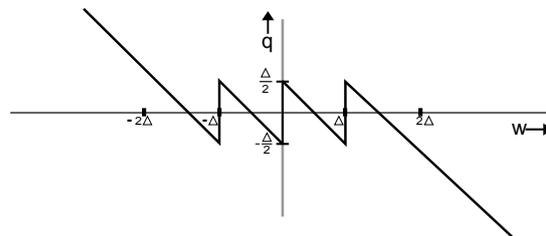
Figure 3.5: Quantization error signal of a two bit midrise quantizer
