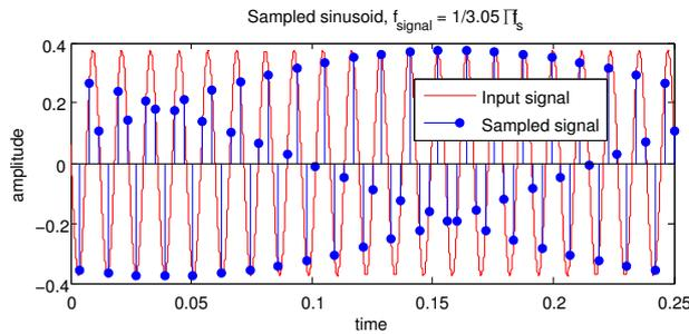
Figure 4.16: Sampling of a sine wave: illustration of variation in short interval estimated PDF. When this PDF is estimated for example from 0 to 0.1 seconds and from 0.1 to 0.2 seconds, the resulting PDFs will be different.
