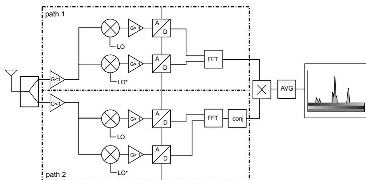
Figure 2.7: Quadrature mixing FX cross-correlation spectrum analyzer (LO\* denotes the 90 degrees shifted oscillator signal phase)
