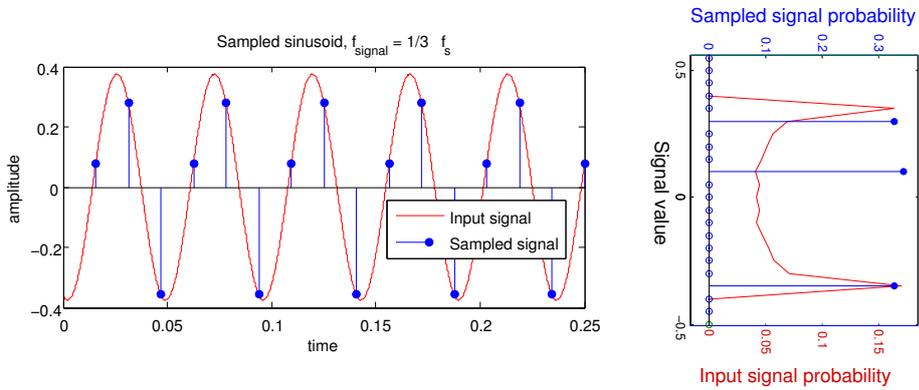
Figure 4.15: A sampled sine wave and its non-symmetrical PDF of a sampled sine wave.
