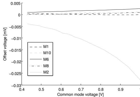
Figure 5.9: Common mode dependent offset for 5nM difference in MOSFET length for components shown in figure 5.2.
