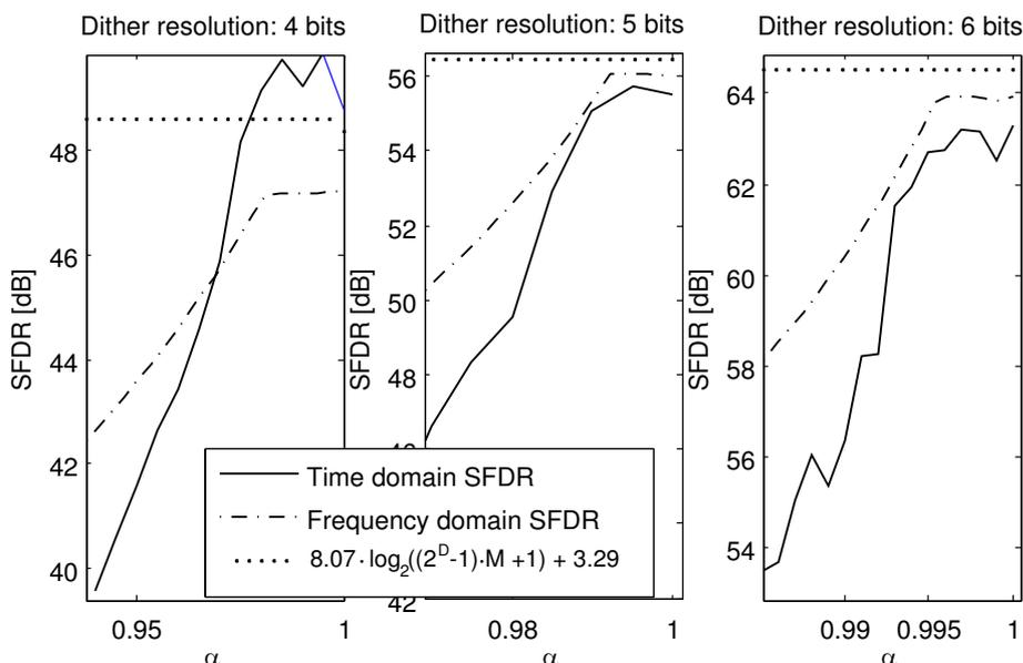
Figure 3.28: SFDR as a function of  $\alpha$ . The x-axis range is 1 LSB.
