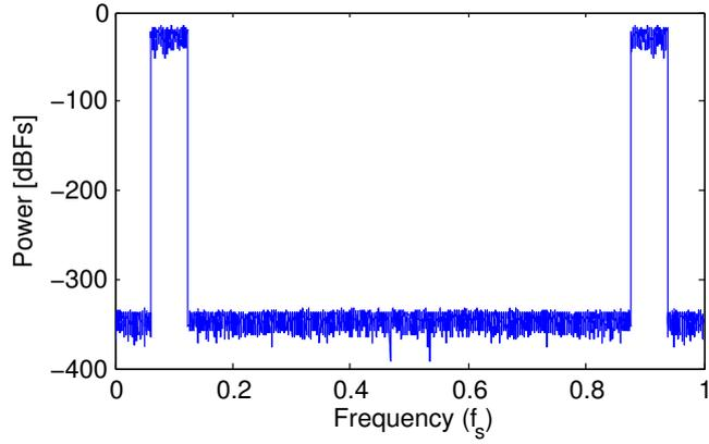
Figure 4.13: Gaussian distributed band-limited input signal.
