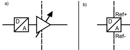
Figure 4.11: Scaling the dither while converting to analog domain. b) is the proposed implementation of a)
