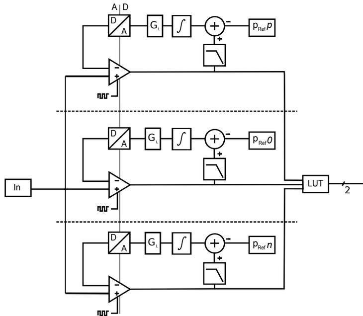
Figure 4.8: Total ADC consisting of three decision level loops
