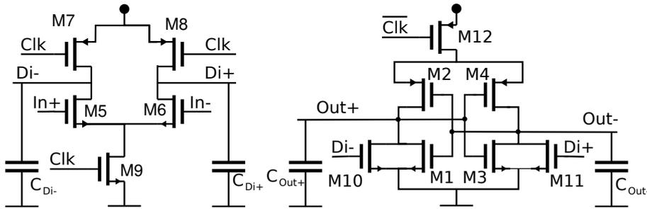
Figure 5.2: Comparator with parasitic capacitances.
