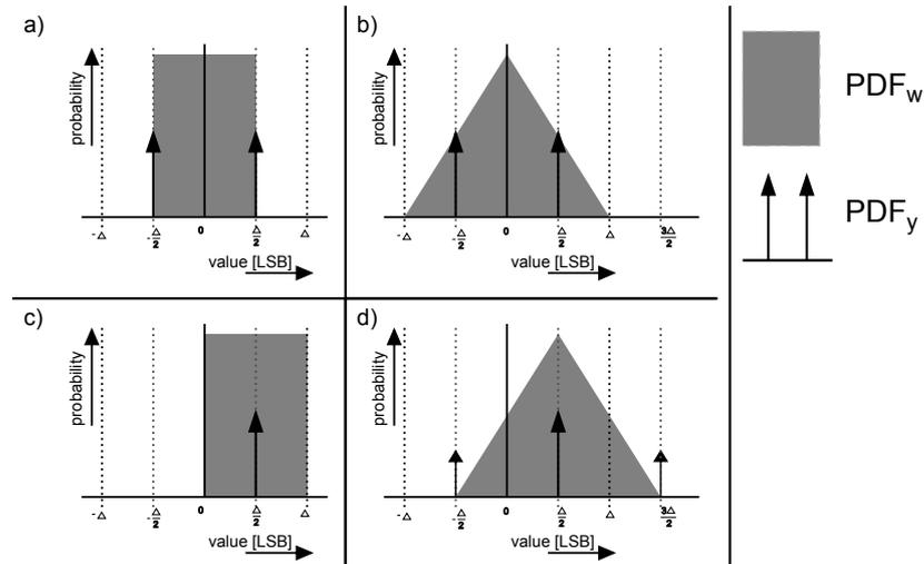
Figure 3.14: Illustration of dependency of total error power on input signal. For rectangular dither the total error power depends on the input signal.
