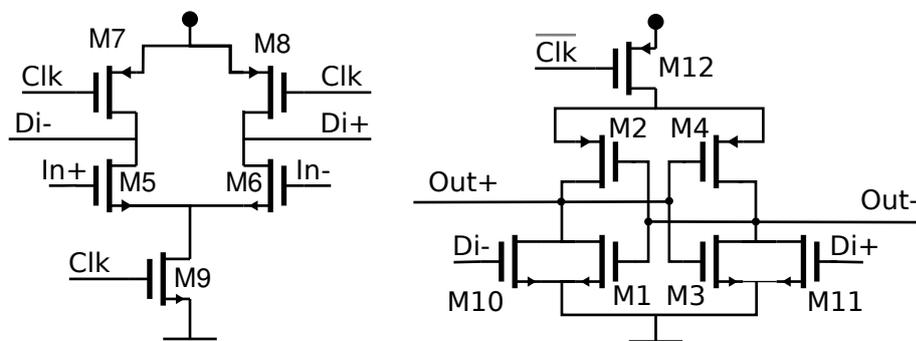
Figure 5.1: Double tail voltage sense amplifier [35], consisting of an input stage (left) and a latch (right).
