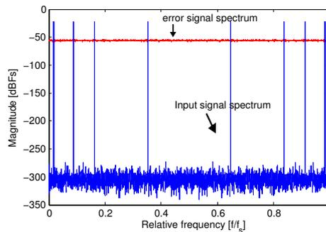
Figure 3.15: Spectra of rectangular dithered signal, consisting of five sinusoids. The signal and total error spectrum are shown.
