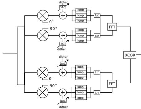
Figure 4.14: ADCs in a total system in case of an FX correlator. Decision level feedback to dither DAC, attenuator and averaging not drawn. For each ADC one dither DAC is introduced.
