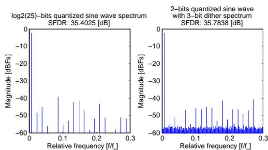
Figure 3.23: Spectra of a  $\log(25)$ -bits equivalent quantizer and the 3-bit rectangular dithered 2-bit quantizer: they have approximately the same SFDR. (MATLAB code in appendix C.3)
