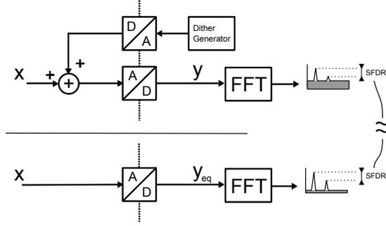
Figure 3.21: Equivalent quantizer resulting in equal distortion component magnitude
