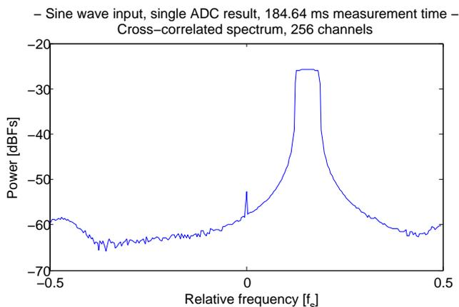
Figure 4.28: Total IF front-end simulation, spectrum (when settled), settings used shown in Table 4.5.
