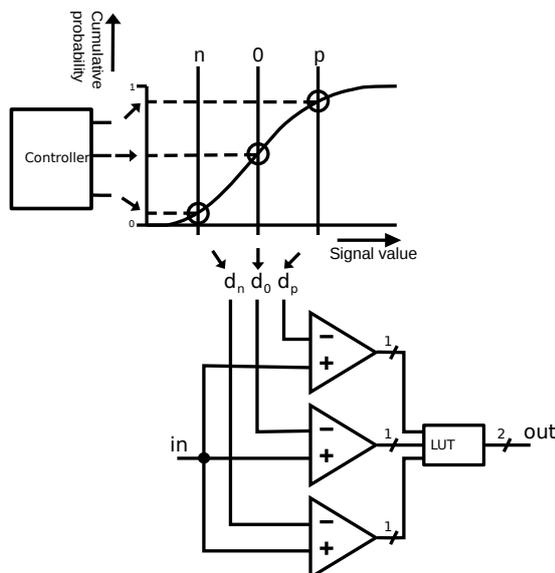
Figure 4.1: Flash ADC with decision levels set through the input signal CDF.
