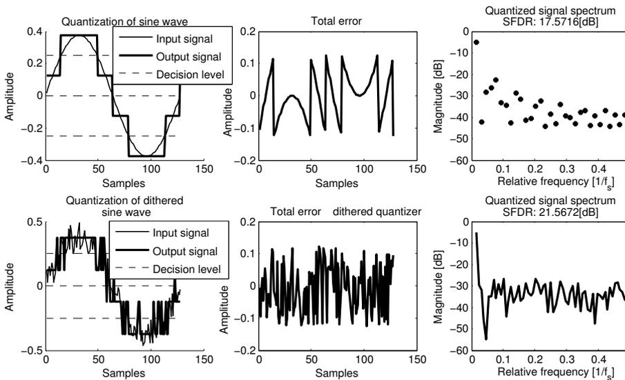
Figure 3.7: Quantized undithered and dithered sine wave with an amplitude of  $\frac{3}{4}$  full scale, the error signal and spectrum. The spectrum of the undithered signal only contains odd harmonics of the fundamental frequency, the spectrum of the dithered signal also has frequencies at even harmonic frequencies.
