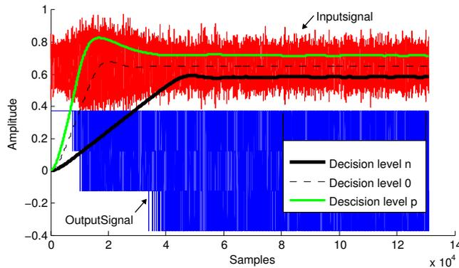
Figure 4.27: Gaussian distributed signal, settling behavior. Settings shown in Table 4.5.
