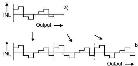
Figure 3.24: Repetitive INL due to INL of dither DAC and quantizer. a) INL of the dither DAC. b) INL of equivalent quantizer.
