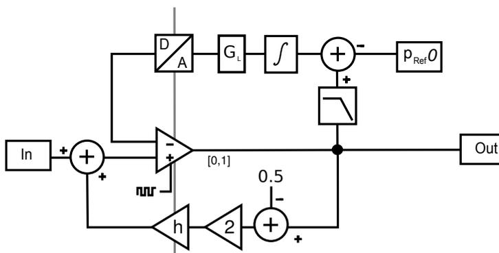
Figure 4.30: Model of decision level loop with comparator with hysteresis effect.
