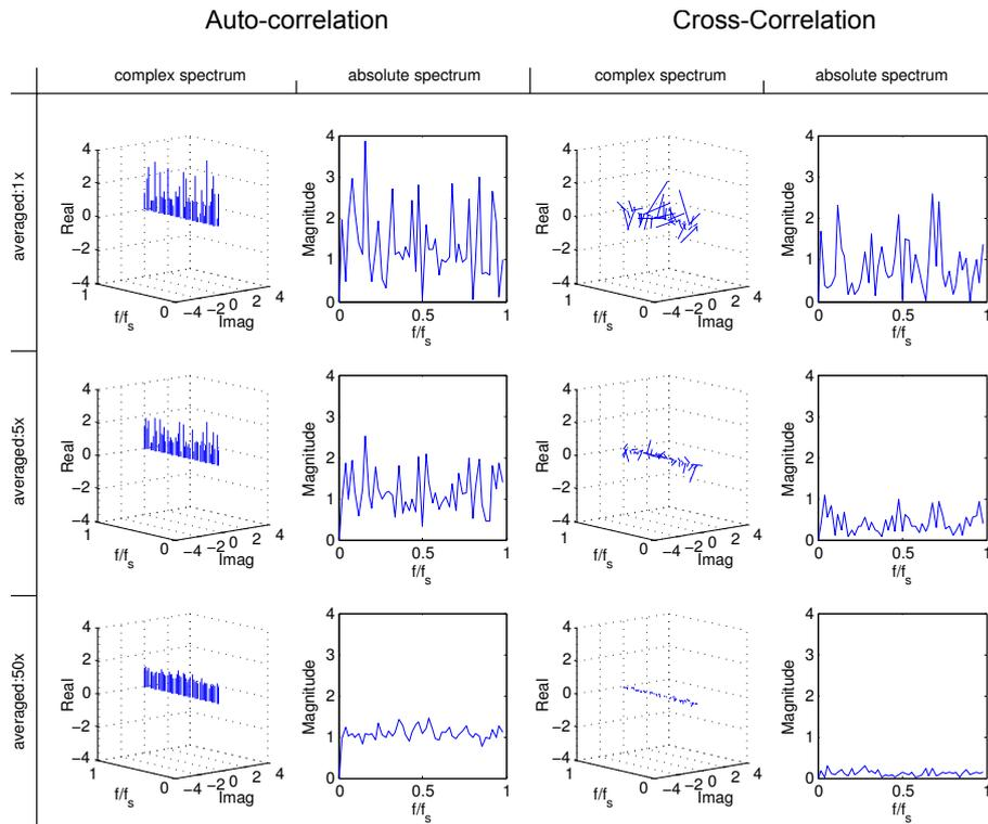
Figure 2.4: Convergence of power spectra when spectrum averaging is applied.
