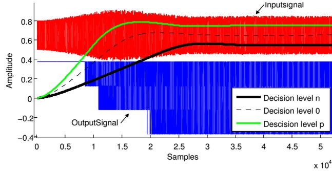
Figure 4.18: Settling of the ADC, settings used shown in Table 4.2. The input signal shown is the input signal at each comparator.
