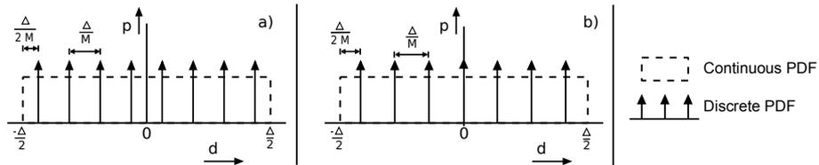
Figure 3.18: Continuous and discrete rectangular PDF dither. a) eight discrete dither values ( $M = 8$ ), b) seven discrete dither values ( $M = 7$ ).
