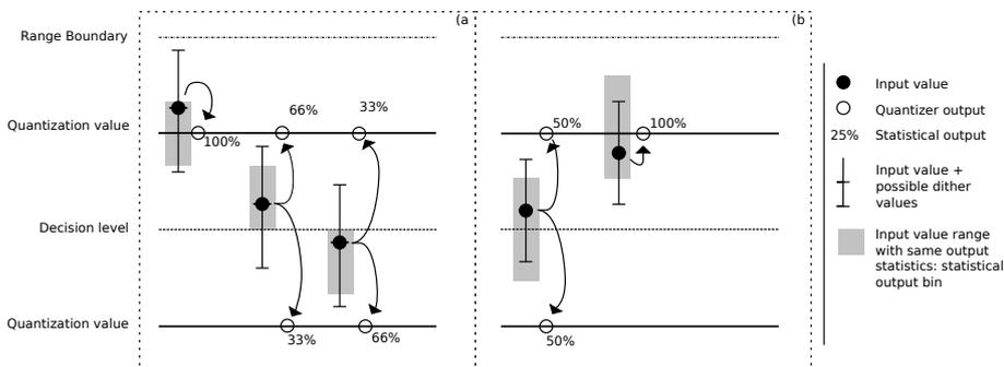
Figure 3.20: Effect of: a) 3 valued dither signals. b) 2 valued dither signals.
