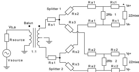
Figure 2.8: Passive splitter [6]
