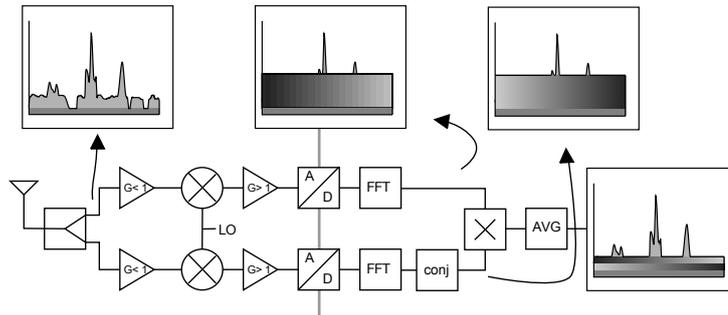
Figure 2.6: Cross-correlation spectrum analyzer
