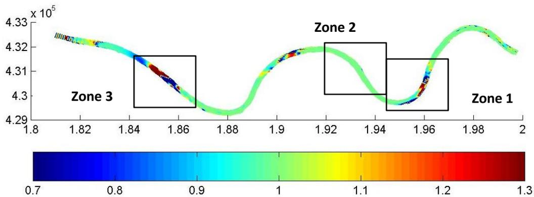
Figure 6.1 Relative cumulative erosion/deposition for the  $\tau_{bio} = 2.85\tau_o$  scenario. Fixed values for visualization purposes
