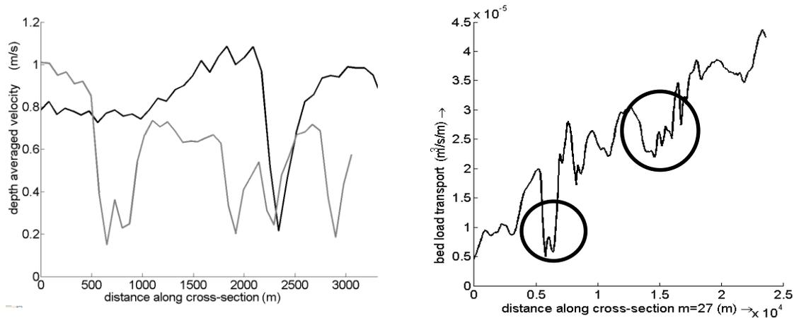
**Figure 6.8** Depth averaged velocity (left) in the northern and southern bend (black line Northern, gray line Southern). Bed load transport (right) along a central line in the navigation channel ( $t=70^{\text{th}}$  month). Fixed rock layers are enclosed.
