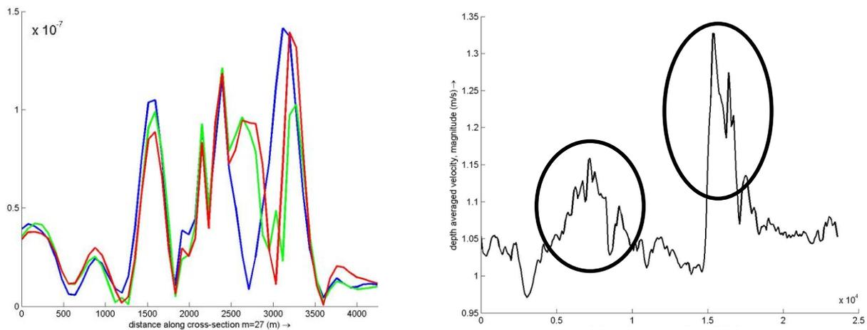
**Figure 6.12** Difference in bed load transport [ $\text{m}^3/\text{s}/\text{m}$ ] after 13 years, with respect the abiotic scenario (left). Depth averaged flow velocity for a center line of the navigation channel (right).  $\tau_{\text{bio}} = 15.9 \tau_o$ ,  $\tau_{\text{bio}} = 2.85 \tau_o$ ,  $\tau_{\text{bio}} = .8 \tau_o$
