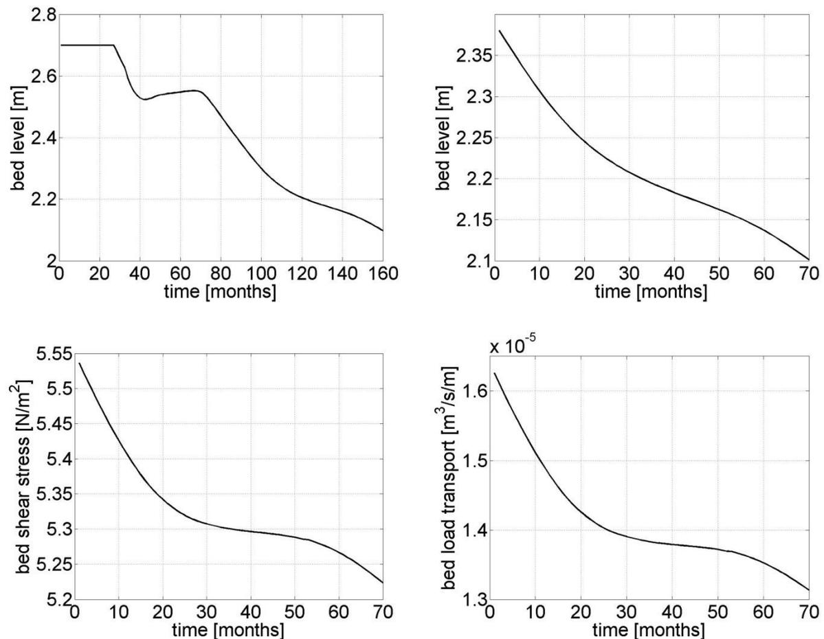
**Figure 6.3** Modeled bed level changes in Zone # 2 for a running period of 13 years (top left). Bed level changes after system adjustments (top right). C) Bed Shear stress (bottom left) and the bed load Transport (bottom right)
