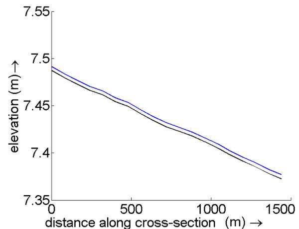
**Figure 6.14** Water levels in zones 1 and 3. Backwater curve caused by the benthic activity in Zone 2 (left), changes in upstream water level (right). The figure only shows the results of the  $\tau_{bio} = 15.9 \tau_o$  scenario because the similarity with other scenarios.
