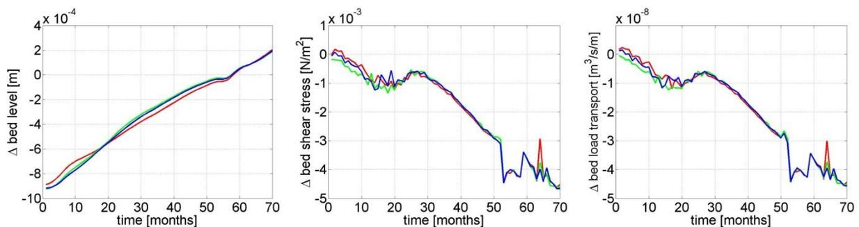
**Figure 6.9** Navigation channel changes in bed level (left), bed shear stress (middle) and bed load transport (right) caused by increase/decrease of the erosion threshold (biotic – abiotic).  $\tau_{\text{bio}} = 15.9 \tau_o$ ,  $\tau_{\text{bio}} = 2.85 \tau_o$ ,  $\tau_{\text{bio}} = 0.8 \tau_o$
