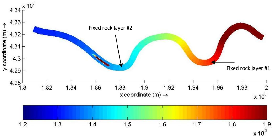
**Figure 5.5** Grain size ( $D_{50}$ ) distribution in the Navigation channel of the River Waal. According to the model provided by Deltares.
