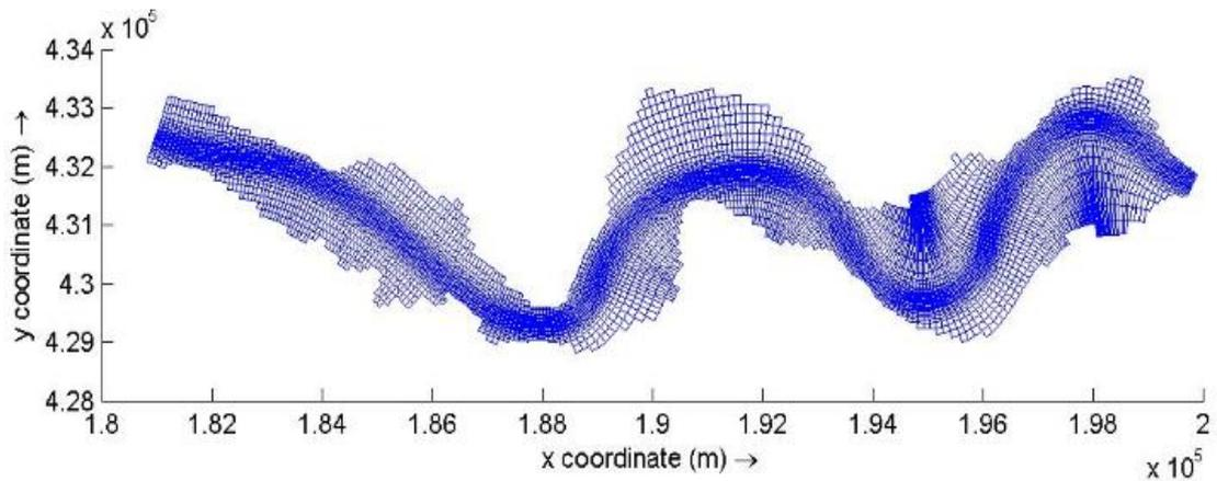
Figure 5.1 Computational Grid of the River Waal (Pannerdenschep Kop - Nijmegen)
