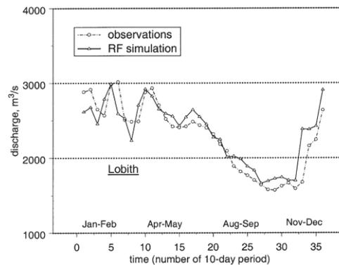
Figure 7.2 Observed discharge of the Rhine at Lobith compared with a simulation (Shabalova et al. 2003)
