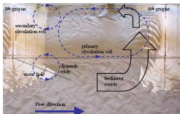
**Figure 6.4** Flow and sediment processes for emerged groynes. (flume experiment) (Yossef and de Vriend 2010)
