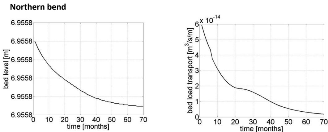
Figure 6.5 Bed level (left) and Bed load transport (right) in the Northern bend of Zone 2
