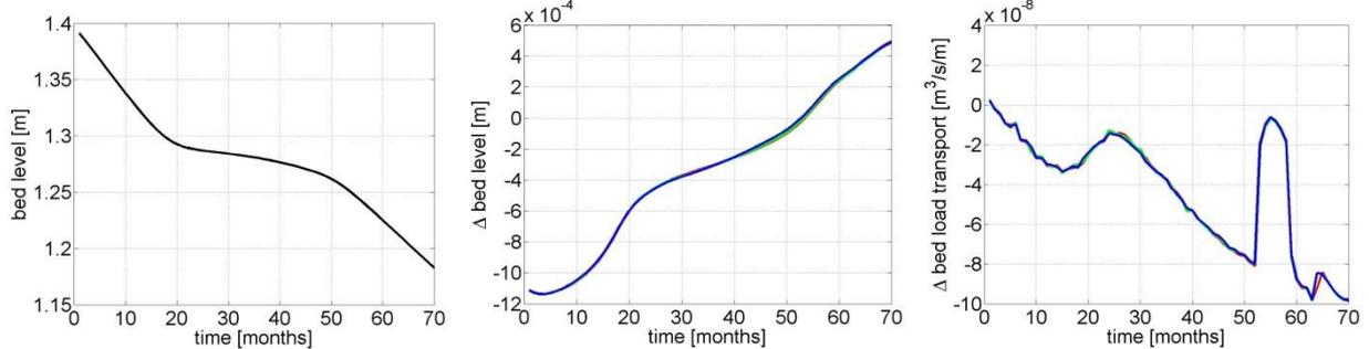
**Figure 6.13** Changes in bed level (left), bed shear stress (middle) and bed load transport (right) caused by increase of the erosion threshold in Zone 1 and 3.  $\tau_{bio} = 15.9 \tau_o$ ,  $\tau_{bio} = 2.85 \tau_o$ ,  $\tau_{bio} = .8 \tau_o$
