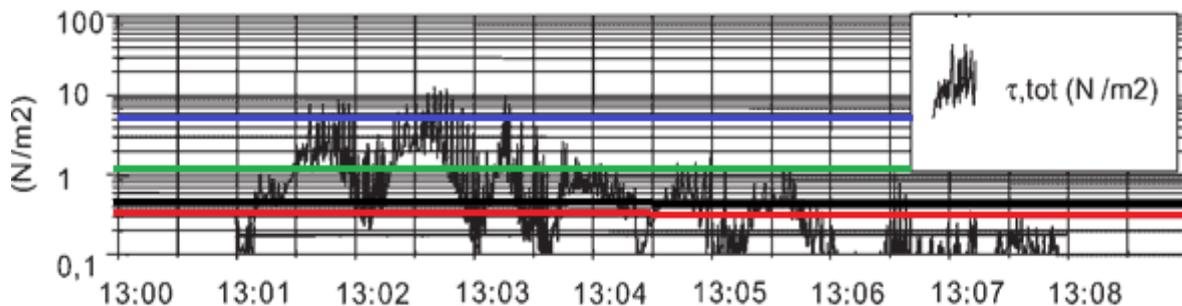
Figure 7.3 Bed shear stress on the south bank, of a straight stretch of a the River Waal, during the passage of a fully loaded motorized vessel (Ten Brinke et al. 2004). Lines:  $\tau_0$ ,  $\tau_{bio}=0.8 \tau_0$ ,  $\tau_{bio}=2.85 \tau_0$ ,  $\tau_{bio}=15.9\tau_0$
