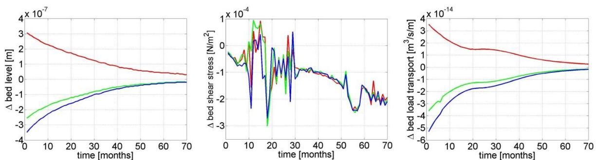
**Figure 6.10** Changes in bed level (left), bed shear stress (middle) and bed load transport (right) caused by increase of the erosion threshold (biotic – abiotic).  $\tau_{bio} = 15.9 \tau_o$ ,  $\tau_{bio} = 2.85 \tau_o$ ,  $\tau_{bio} = .8 \tau_o$
