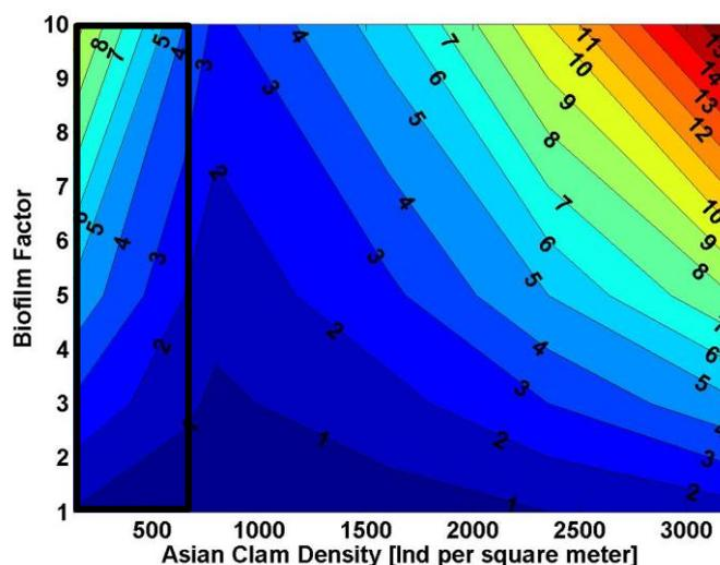
**Figure 4.2** Expected biotic erosion threshold for Asian Clam communities. The rectangle indicates the zone of the current situation (average and maximum densities) in the River Waal ( $\tau_{\text{bio}}/\tau_0$ ).
