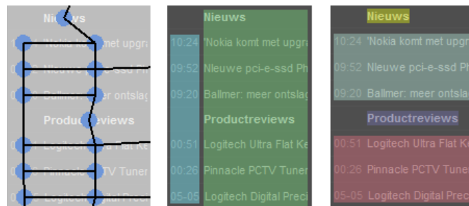
Figure 10: On the left is the grid, the middle shows the problem of selecting the largest block, and the right side is how we would expect it to be.
