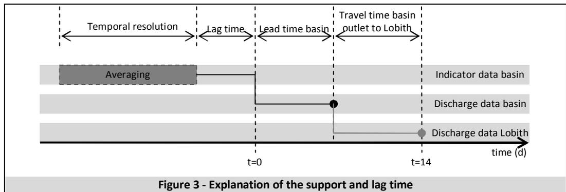
Figure 3 - Explanation of the support and lag time
