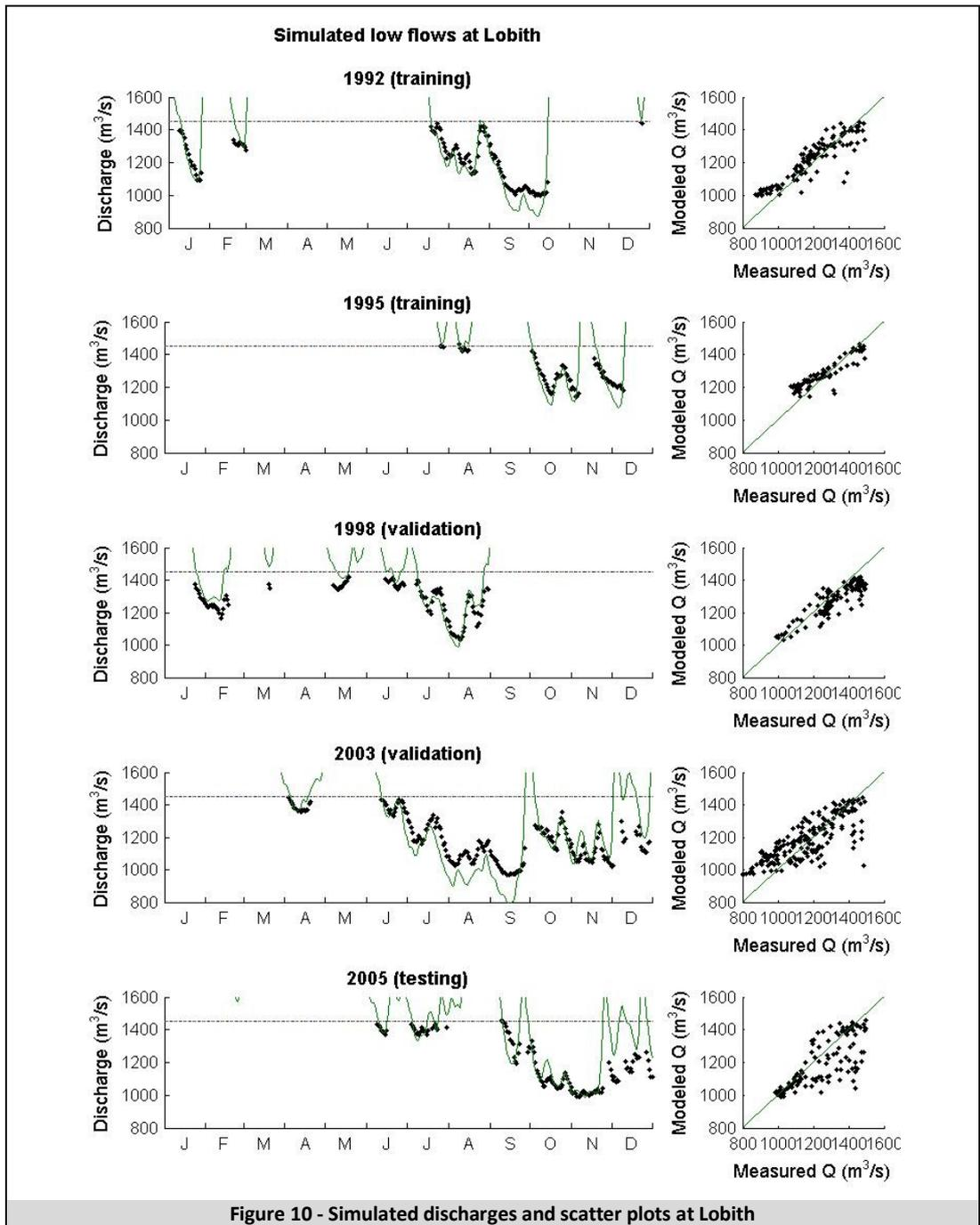
The model error for the sub-basin flows is part of the input of the ANN for Lobith. The ANN for Lobith does not take the error into account, but the Lobith model trains the sub-basin outputs as perfect input. This is a benefit when there is a systematic error in the sub-basin output. If the sub-basin output has a random error, the performances of the test phase could be much lower.
