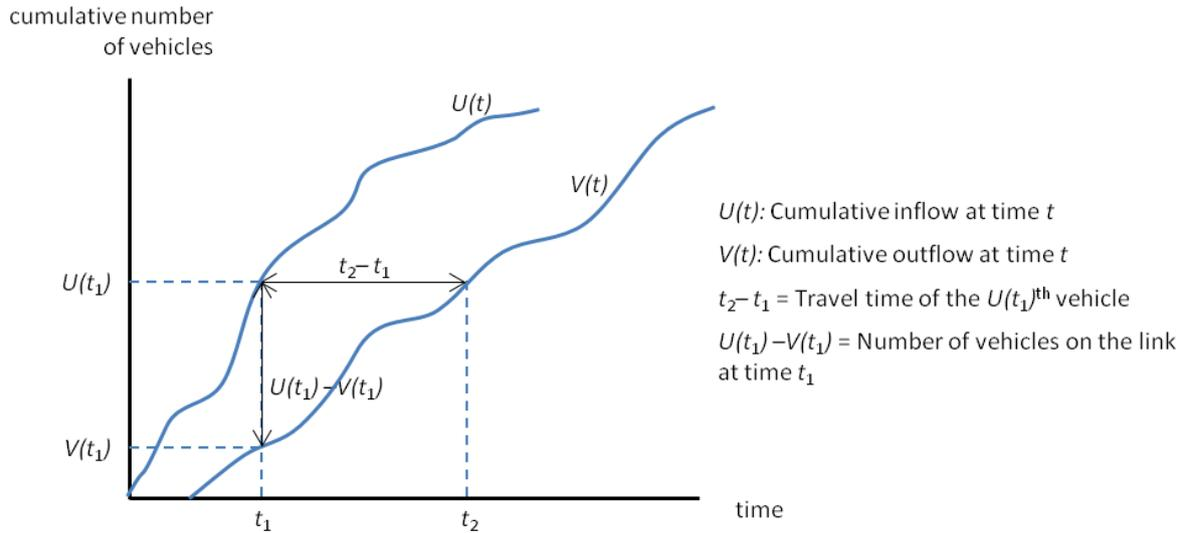
Figure 4. Example of cumulative in- and outflow curves of a link over time.
