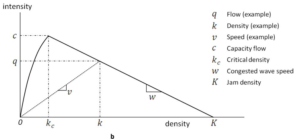
Figure 5. Two examples of a fundamental diagram: (a) Newell's diagram and (b) Smulders' diagram.
