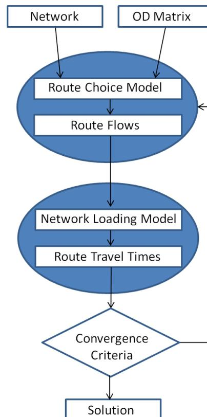
Figure 1. Schematic overview of the traffic assignment model.
