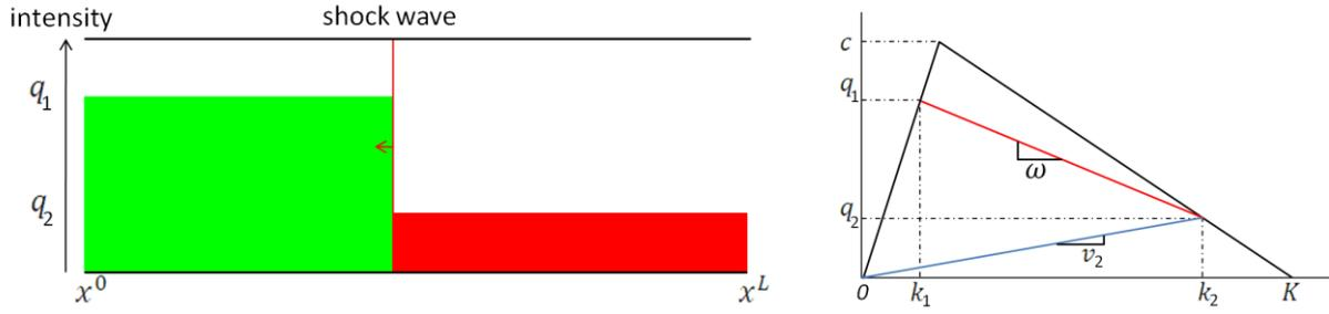
Figure 6. Example of a backward shock wave, with its associated fundamental diagram.
