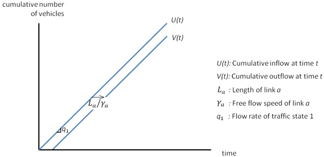
Figure 8. Cumulative vehicle numbers within free flow conditions.
