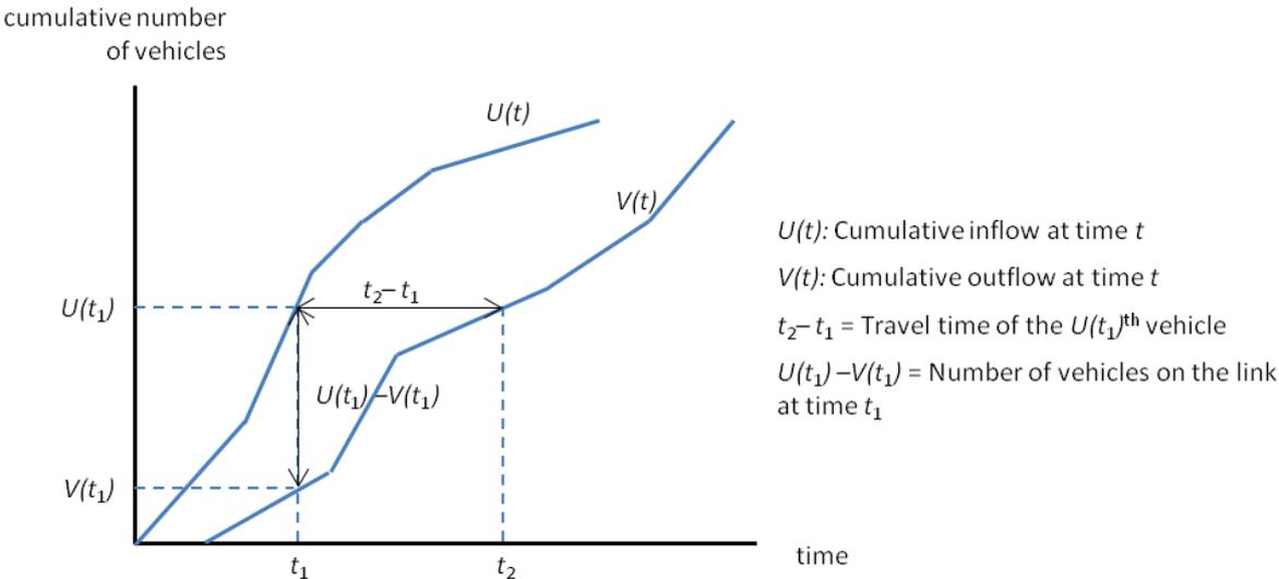
Figure 13. Example of cumulative in- and outflow curves of a link over time.
