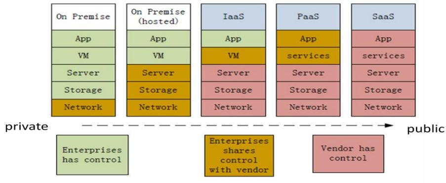
Figure 4 Control Level of Cloud computing (Guo, et al., 2010)
