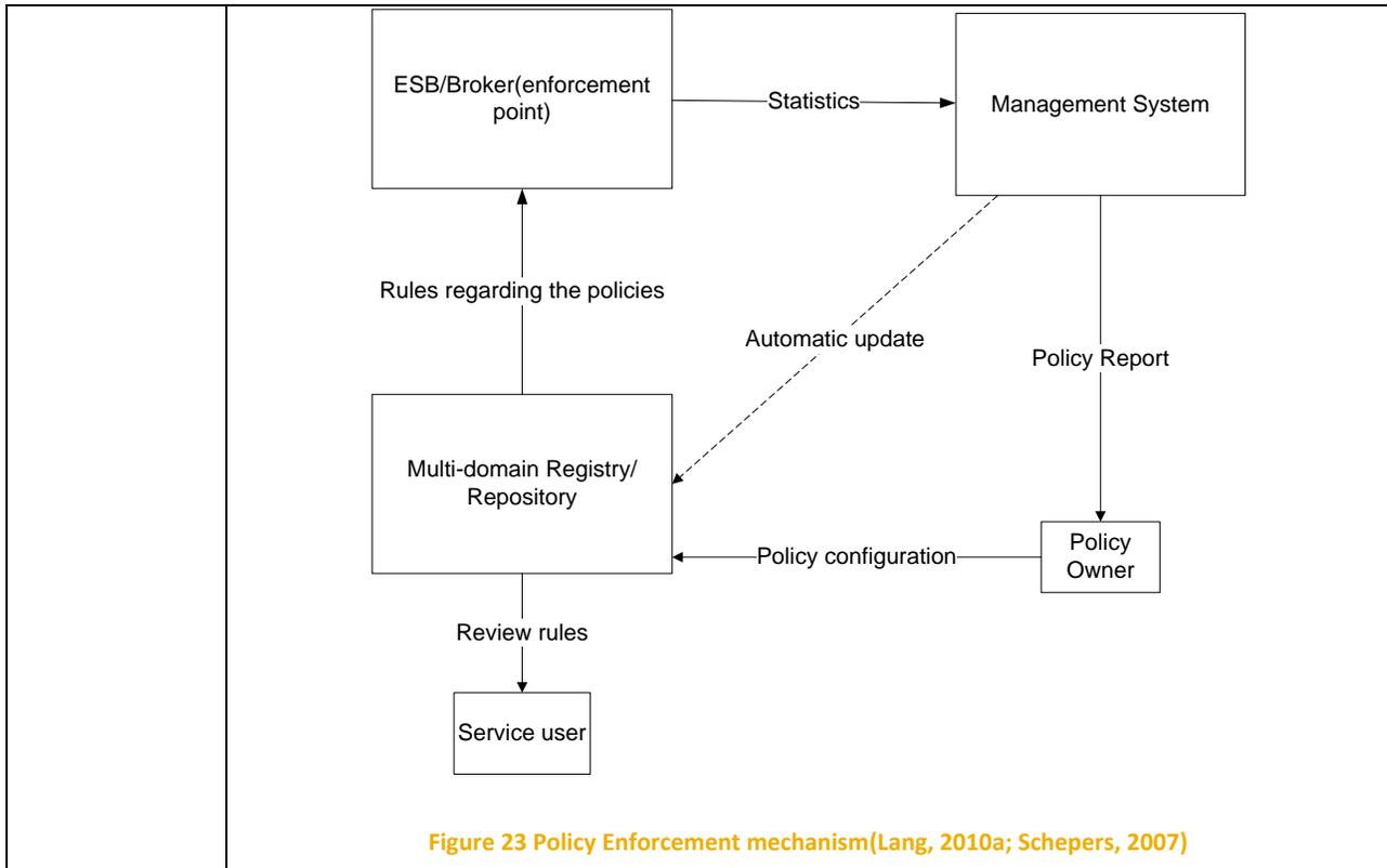
Figure 23 Policy Enforcement mechanism(Lang, 2010a; Schepers, 2007)
