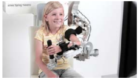
Figure 10.4 A promotion picture of a girl using the Armeo Spring Paediatric, a device guiding movements using gravity compensation and providing feedback with several games shown on a display
