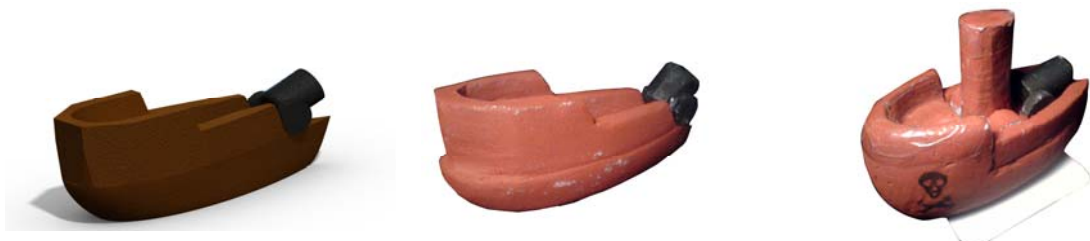
Figure 8.6 3D-model of new version of boat, realisation of boat and the photo of changed boat (the one used in the tests)
