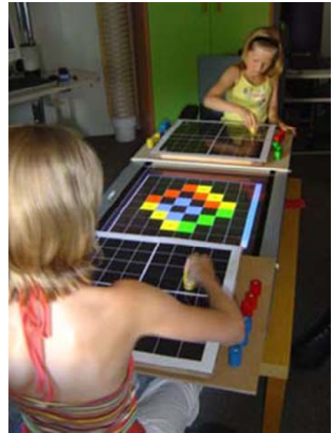
Figure 3.2 The first version of the TagTile consisting of three parts: in the middle there is a plasma screen and at both ends a 8 by 8 sensor grid.
