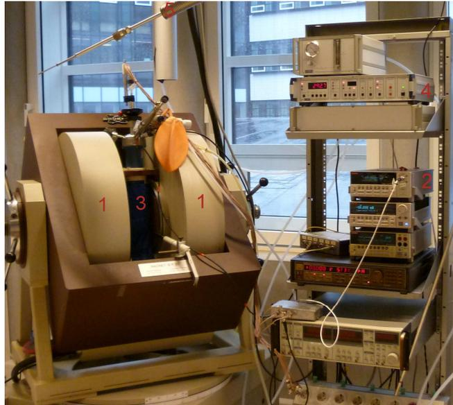
**Fig. 4.1.1:** Photograph of the “Bruker” system. Among its constituent parts are an electromagnet (1), measurement electronics (2), a cryostat containing the sample (3), a temperature controller (4) and a connection to an external helium vessel (5).
