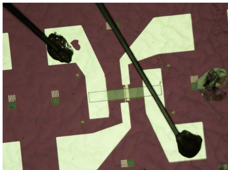
**Fig. 3.5.2:** A device bonded by using silver epoxy. Note that the hole in the upper left contact pad was already pre-existent and does not protrude into the SiO<sub>2</sub> layer. The damage in the right part of the image is caused by breaking a wire at the substrate.
