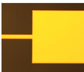
**Figure 30.** Optical microscope image of a template-stripped Au electrode embedded in PMMA; the PMMA was cooled down slowly after spin-coating and baking at 120°C and the UV-curing time was reduced.
