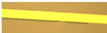
**Figure 18.** Optical microscopy image of an Au electrode after metal lift-off in acetone overnight; at the edges of the electrode contaminations of remaining resist can be seen.
