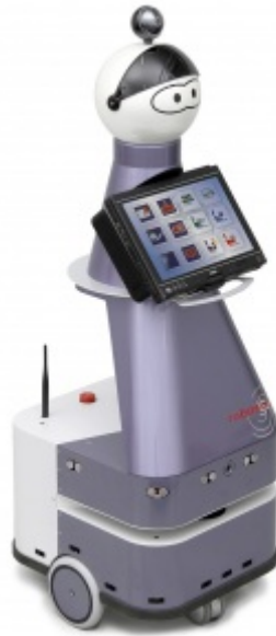
Figure 2.2.: An assistive robot called Kompai by Robosoft (Robosoft, 2010)
