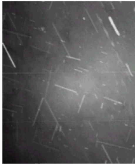
Figure 3-32: {311} Type defects for the weak beam dark field imaging condition 19 .
