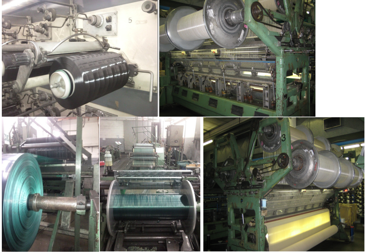
Figure 5 – (semi)-finished products; Top left – a wounded bobbin; Top right – a knitting machine with beams on top; Down Left – a wounded monotape roll being stretched; Down centre – a beam in process in the stretching department; Down right – a knitted roll being manufactured.
