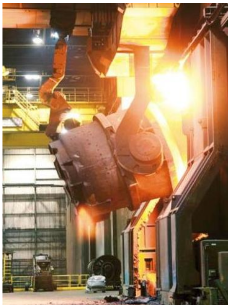
Figure 3.1 - Pig iron is poured into a converter
