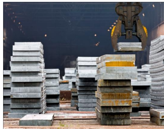
Figure 3.11 - Overhead gantry crane picks 2 slabs from a stack and brings them to the RS
