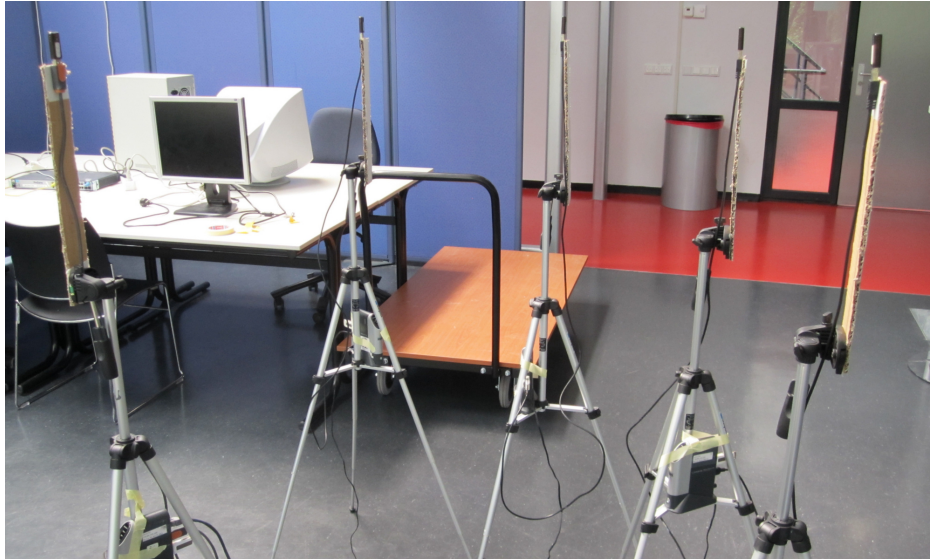
Figure 7.3: Photo of the measurement setup used to find the optimal dongle orientation.
