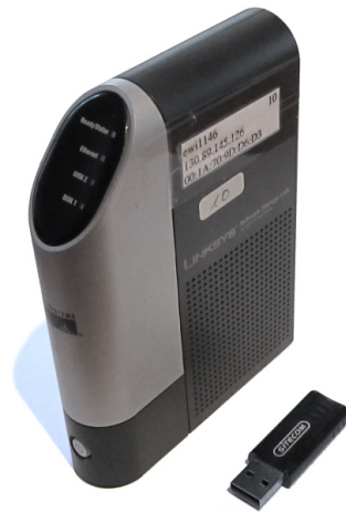
Figure 3.3: Linksys NSLU2 device and Sitecom CN-512 v2 001 Bluetooth dongle
