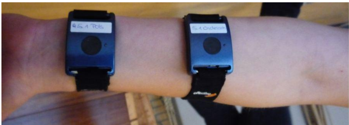
Figure 3.2.1. Wearable EDA Affectiva Q™ Sensor curve attached to the wrist and forearm.
