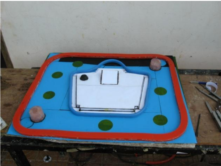
Fig. 14 - Hand-layup mold SHS back part
