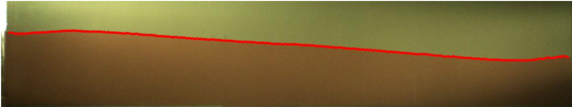
Figure 6.2: Example of analysis of a frame in a numerics verification experiment. The red line indicates the location of the water surface as found by the analysis program.
