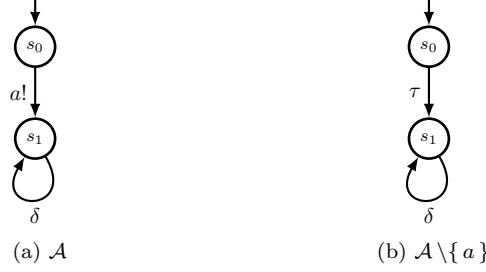
Figure 3.6: Well-formed QTSs are not closed under action hiding if states with internal transitions are considered quiescent.
