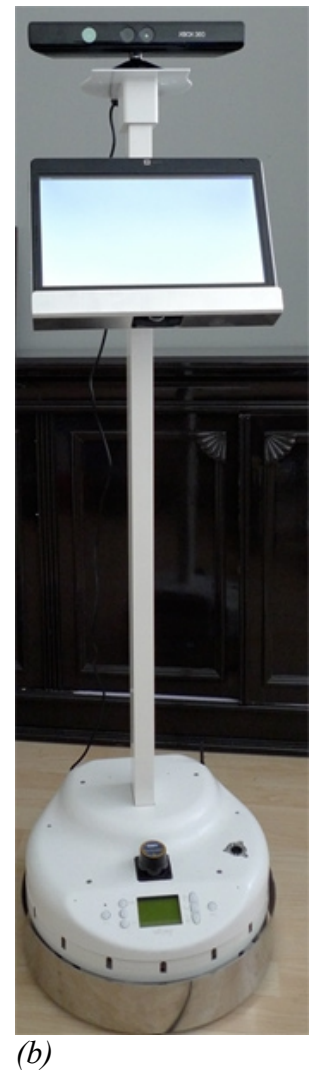
Figure 2: Florence Robot. (a) Tablet-PC with robot face, (b) Wany Pekee PC base with stand, Tablet PC, and Kinect sensor.
