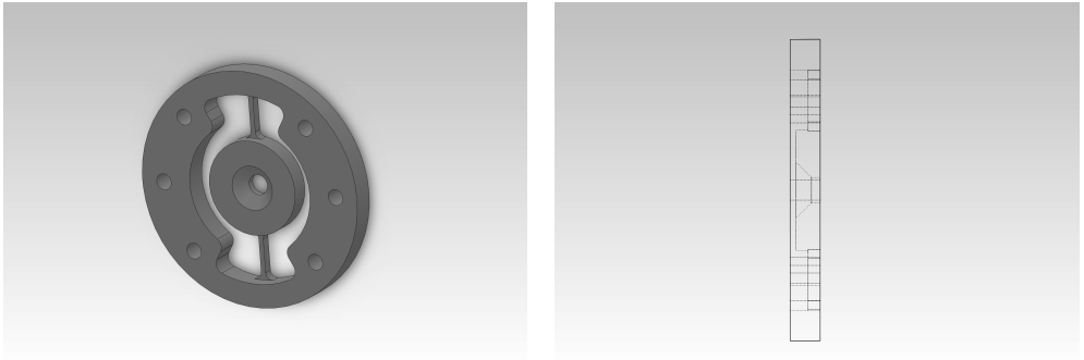
Figure 4.5: The final design of the torque sensor. Left the dimetric view is shown, right the side-view.
