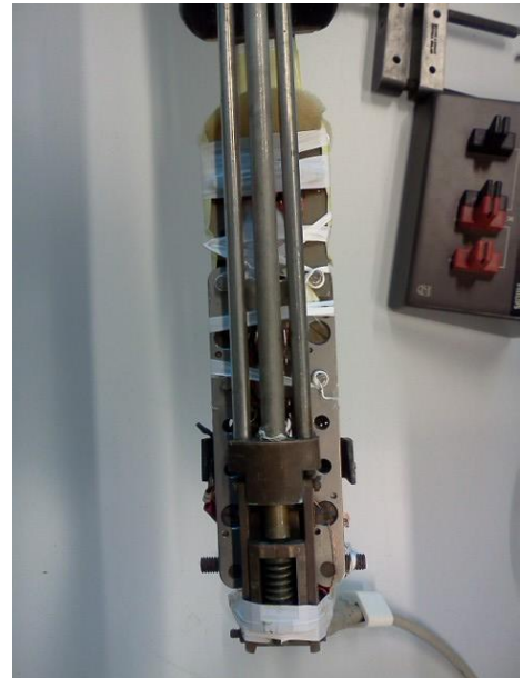
Figure 10 Photo of the U-shaped sample holder
