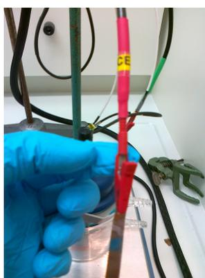
**Figure C.2:** Connecting the Counter Electrode
