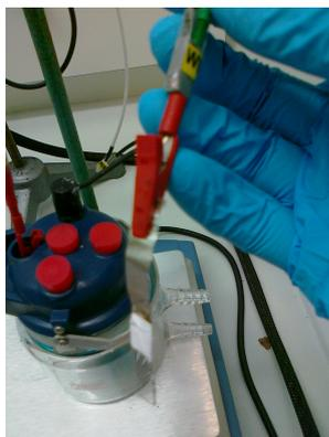
**Figure C.3:** Connecting the Working Electrode
