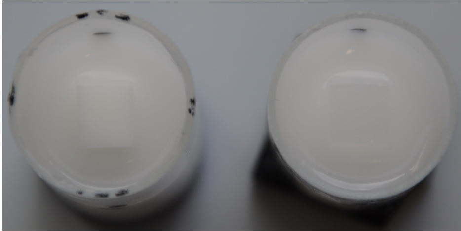
Figure 2.4: Unfinished phantoms, to the left with a high \mu_s' inclusion, to the right with a low \mu_s' inclusion.
