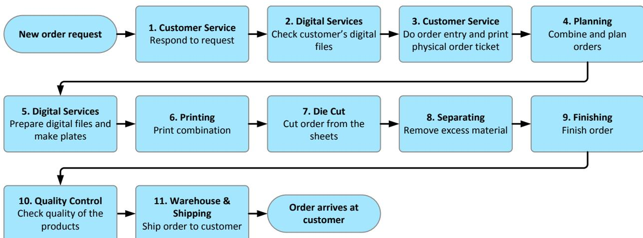
**Figure 7: General manufacturing process at AVDS.**
