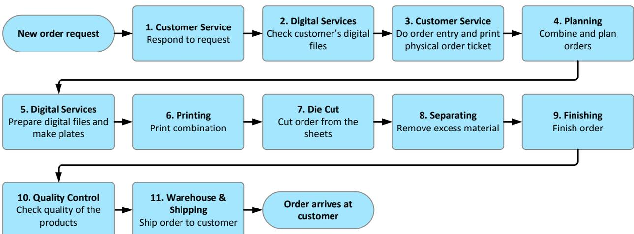
**Figure 7: General manufacturing process at AVDS.**
