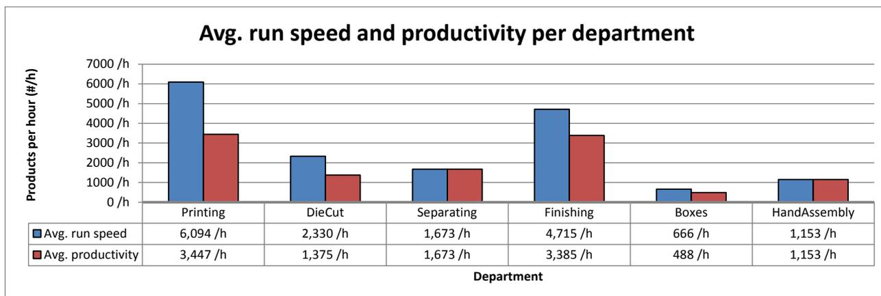
**Figure 19: Average run speed and productivity per department during Q1 of 2012.**
