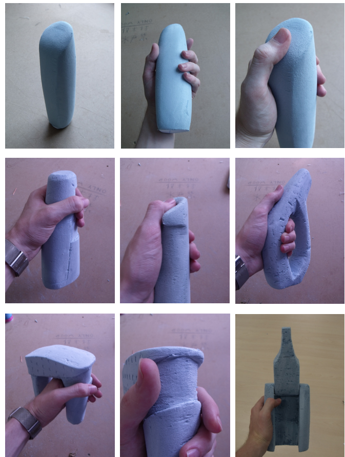
Figure 3.5 Various shape models which were constructed to verify ideas and gains insight in the constraints of the design.
