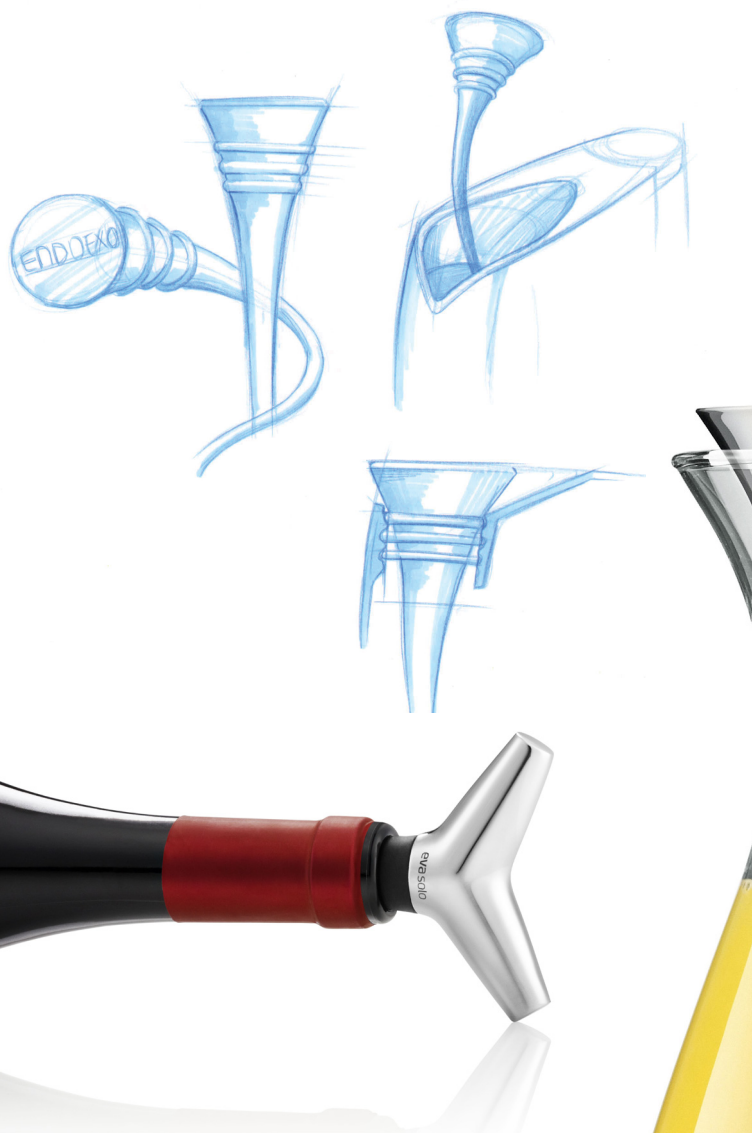
Figure 4.11 (Below) Design sketches for the water plug which was inspired by wine stoppers of Eva Solo and Silit and bathroom sink stoppers.
