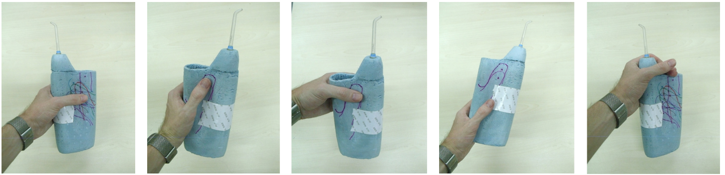
Figure 3.9 The design of this shape model does not instruct the user clearly in how to hold and operate it.
