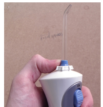
Figure 3.8 The arm (distance) between the point of mass of the water reservoir and the wrist joint is larger, therefore the user is strained more, and the design becomes unstable.
