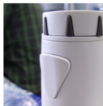
Figure 4.22 The surface of the jet tip release button is not smoothly curved.
