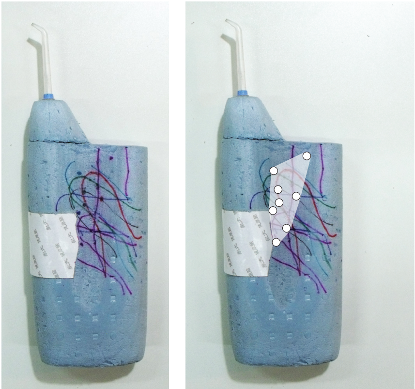
Figure 3.10 Giving some indication into where the activation button was placed made the more understandable how to hold the product. However, the pressure point of thumb still varied between different testing subjects.
