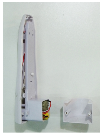
Figure 2.16 (Above) Assembly of the Candeon utilizes hook and screw connections.
