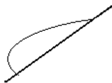
Figure 6: Exaggerated picture of a droplet on a skewed surface. As can be seen, more liquid is on the lower end of the surface.
