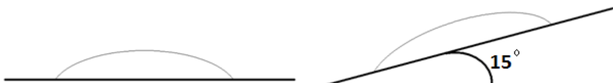
Figure 8: Schematic drawing of the drying of the samples. One sample is just lying flat, while the other is drying under an angle of 15°.
