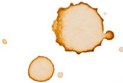
Figure 1: Some coffee stains, which have a distinctive darker color on the perimeter, suggesting higher concentrations of particles there.
