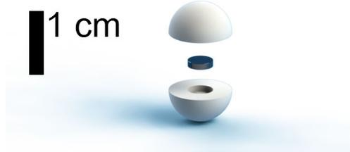
Figure 3.2: Illustration of a sphere with a diameter of 10 mm and a magnet of 4 mm diameter and 1 mm thickness. Exploded view.
