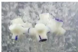
Figure C.9: Five tetrapods fitted with 5 mm magnets and 5.5 mm caps forming a pentamer at an airflow of  $52.4 \text{ cm}^3/\text{s}$ . Although it seems to be a ring-like structure, it is not because the chain is not closed. This is a structure without defects and thus useful for the formation of crystal structures
