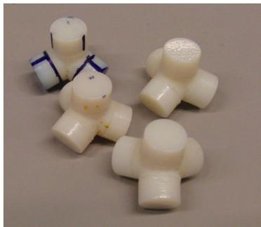
Figure 3.5: Photograph of tetrapods as used in this thesis. The tetrapods shown are fitted with 5 mm diameter neodymium disk shaped magnets and 5.5 mm caps.
