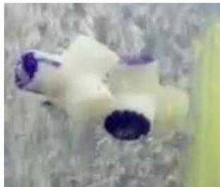
Figure C.2: Two tetrapods fitted with 5 mm magnets and 5.5 mm caps forming a dimer with three pods of both tetrapods pairing with each other at an airflow of  $52.4 \text{ cm}^3/s$ . This is a structure with a defect.
