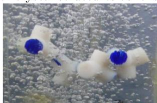
Figure C.7: Four tetrapods forming a tetramer which has a chain structure at an airflow of  $52.4 \text{ cm}^3/\text{s}$ . One tetrapod is placed with a different orientation. This is a structure with defects.
