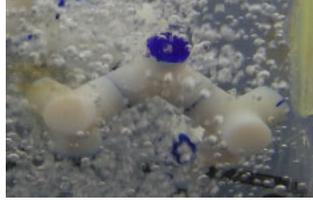
Figure C.3: Three tetrapods fitted with 5 mm magnets and 5.5 mm caps forming a trimer at an airflow of  $52.4 \text{ cm}^3/\text{s}$ . The structure shown is a chain and is useful for the formation of crystal structures as there are no defects in the configuration.
