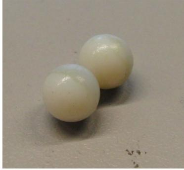
Figure 3.3: Photograph of the spheres with a diameter of 10 mm and a magnet of 4 mm diameter and 1 mm thickness.
