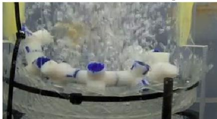
Figure C.11: Eight tetrapods fitted with 5 mm magnets and 5.5 mm caps forming an octomer at an airflow of  $52.4 \text{ cm}^3/\text{s}$ . Several defects are shown. The diameter of the innertube only allows the chain like structure to curl around its curvature, indicating the system is too small.
