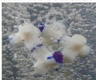
Figure C.8: Four tetrapods forming a tetramer having a ring like structure at an airflow of  $52.4 \text{ cm}^3/\text{s}$ . This is a structure with defects.
