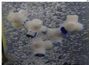
Figure C.10: Five tetrapods fitted with 5 mm magnets and 5.5 mm caps forming a pentamer at an airflow of  $52.4 \text{ cm}^3/\text{s}$ . Several defects occurred in the formation of this pentamer.
