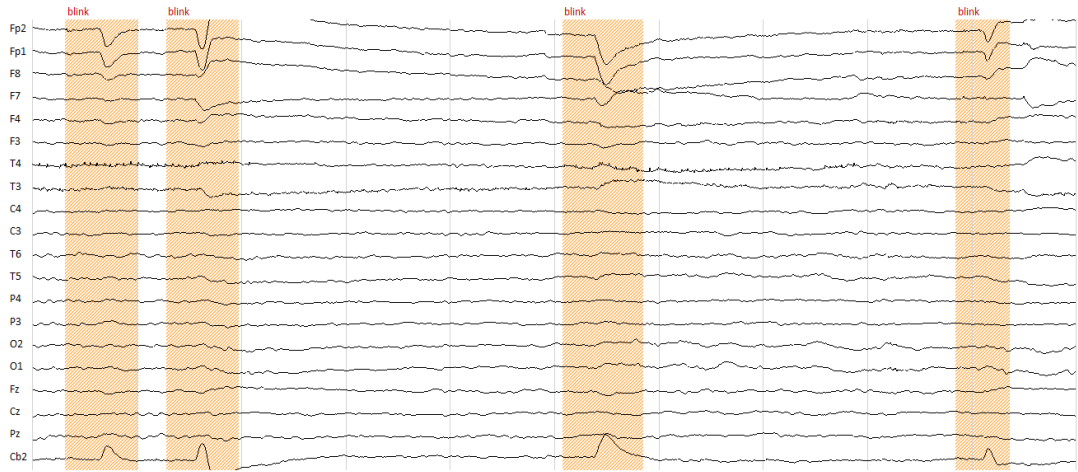
Figure 2.8: Referential montage showing transients caused by eyeblinks (marked parts). We clearly see a correlation between the transient behaviour in channels Fp1 and Fp2 and the EOG-channel (in this file named Cb2).
