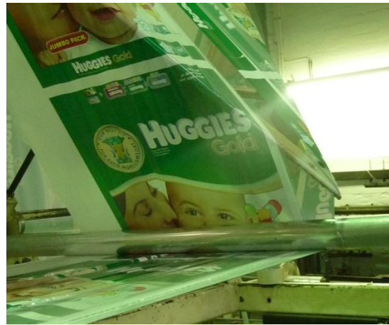
Fig 9.2 – Torn material on the A-frame folder
