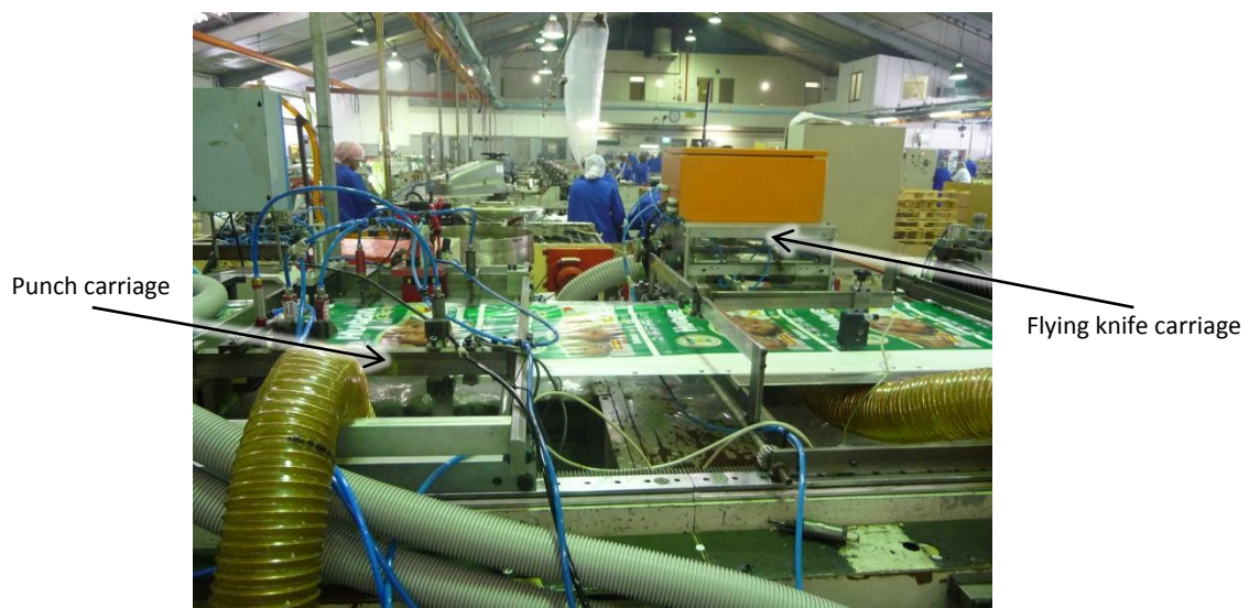
Fig. 10.1 – Flying knife carriage and punch carriage on machine C20
