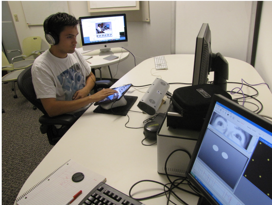
Figure 5.11: Overview of the test set-up, including eye-tracker monitor and recording equipment.
