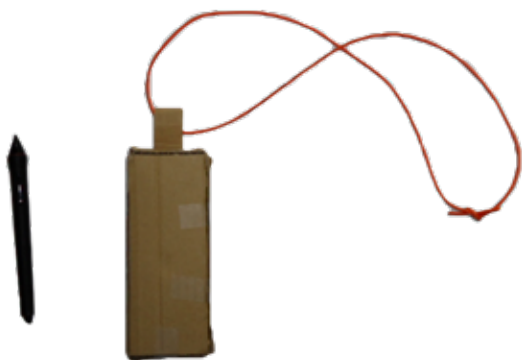
Figure 8.7. A wacom pencil is used to test whether how well a pencil with buttons would work.
