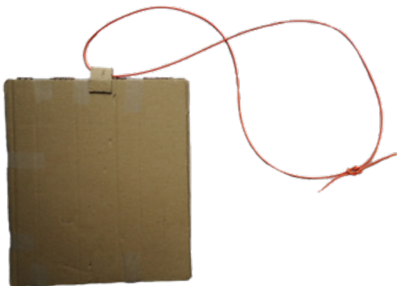
Figure 8.2. A simple carbon plate with iron in it is used to simulate a tablet PC.
