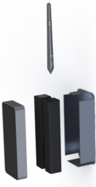
Figure 9.2. A casing holds together the Leap, the pencil holder and the microphone.
