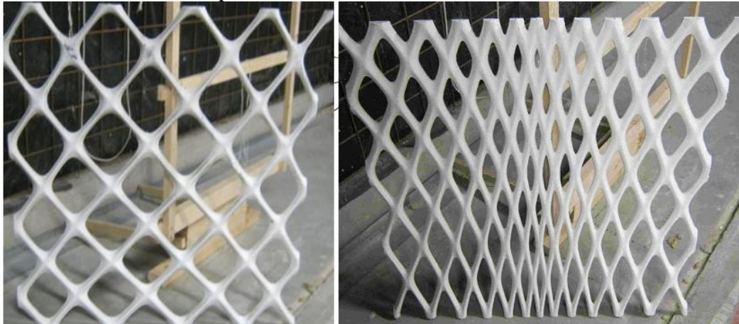
FIGURE 22: TWO STUDIED SAMPLES OF THE MESH. LEFT: PANEL A – MESH WITH MODERATE TRANSPARANCY. RIGHT: PANEL B – MESH WIT LIMITED TRANSPARANCY
