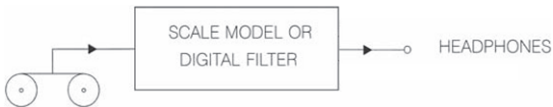
FIGURE 15: THE PRINCIPLE OF AURALISATION
