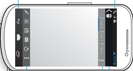
**Action Bar** Available Tabs for navigation, displays current tab with indicator and tab stack overflow. Also the application icon to the left with the up button can exists in the action bar.
