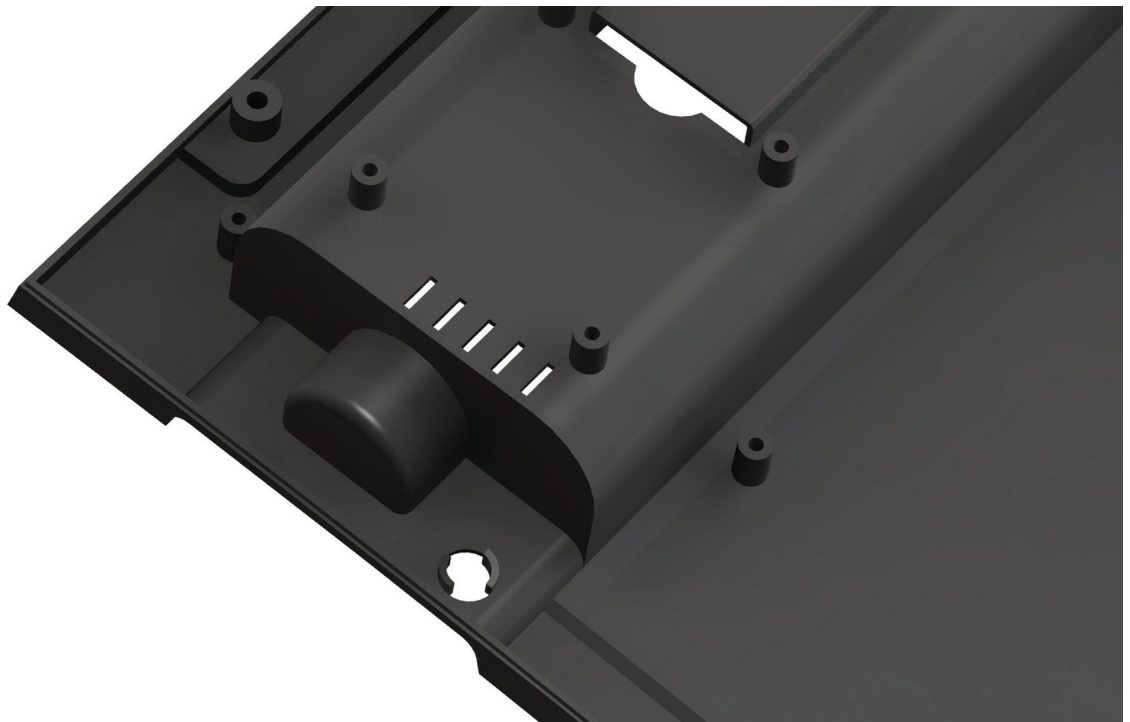
B.05 Details of the battery and SD card container. Buses for assembling the extra PCB with SD card connection and battery connection are also featured. The outer edge has an inner lip for a smooth connection.
