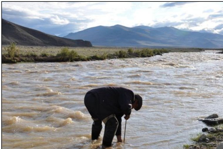
Figure 11 Mr. H. Bagdad, gauging man doing measurements in Chigertei river at Deluun gauge in June, 2011 (IMH Mongolia)
