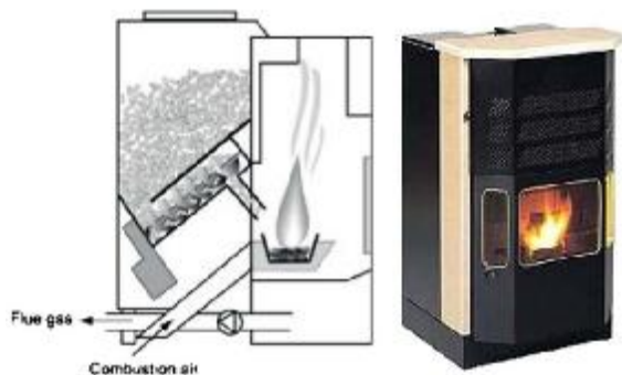
Figure 4 - Boiler with an integrated fuel store
