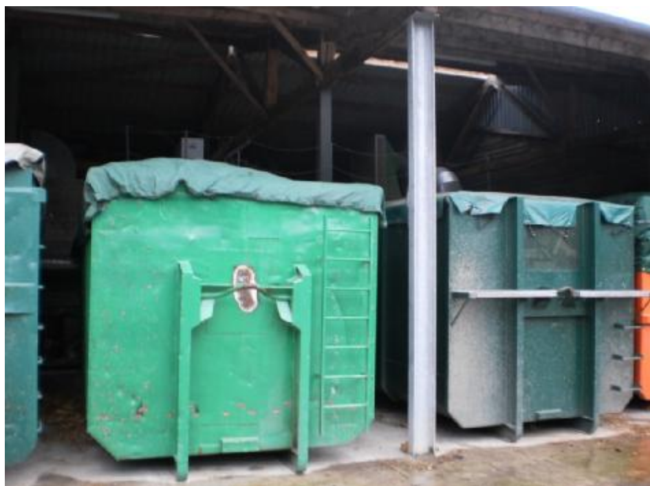
Figure 2 - Residual heat from a biogas installation is used to dry wood chips
