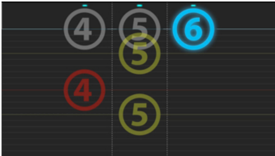
Fig.8 Example of the video-guide for the operator to produce the right movements and rotations. In this particular example the guide is telling the operator to press the key “6”, and to get ready to press they key “5” as well. There were a total of 21 steps, for the operator to anticipate the movement.
