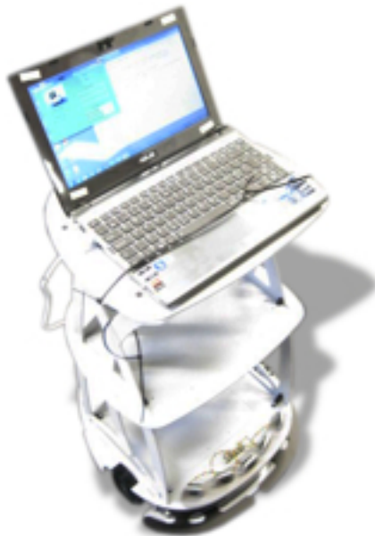
Fig.7 Image of the Magabot robot without the shell. The speakers were placed on the lowest shelf.
