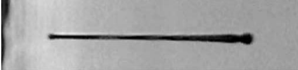
Figure 5: Image of a droplet captured with a LED as illumination displaying motion blur. [6]
