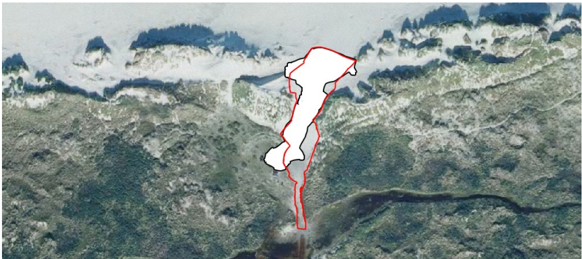
Figure 66: Observation (red) and simulation by XBeach (black) overwash occurring during the Allerheiligenstorm.
