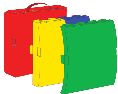
Figure 4.12 : Concept 3, the modules can be clicked on/ off easily.
