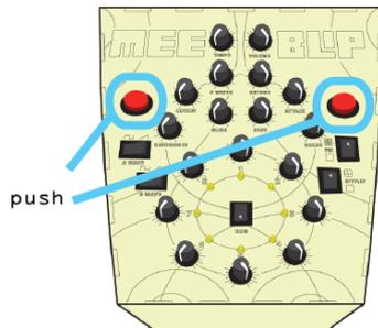
5b) Play automatically using the run switch
