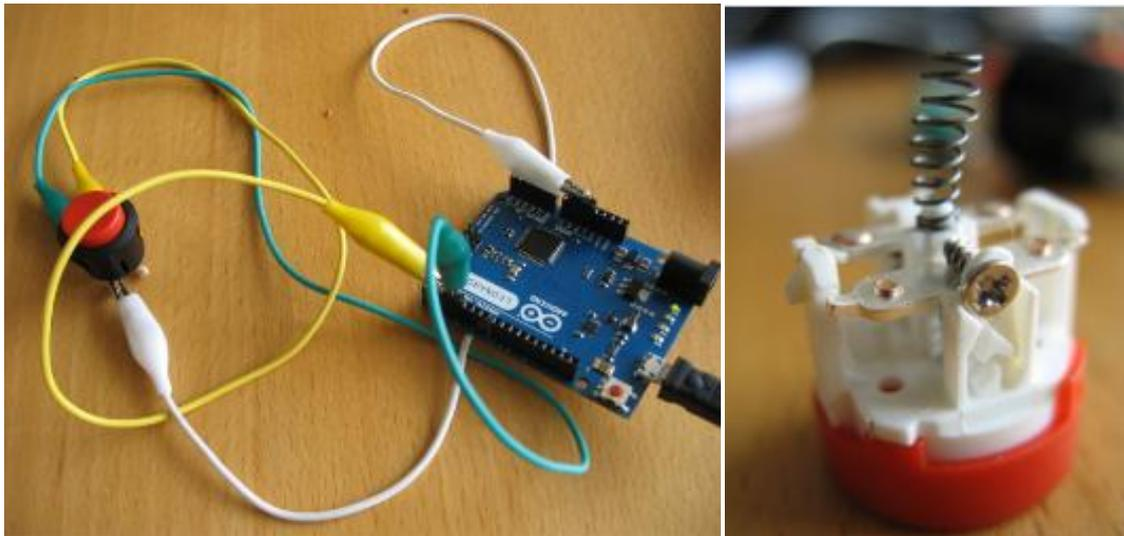
FIGURE 42. ATTEMPT MADE AT VELOCITY SENSITIVE ARCADE BUTTON
