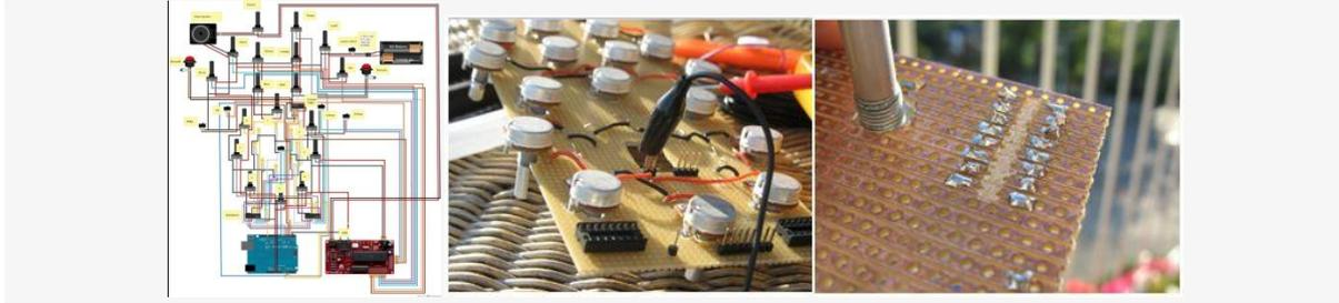
Getting the electronics right in this project is by far the hardest task in this project. If you can make a PCB, go for it, as it will save a lot of time fixing minor errors. Otherwise, use a stripboard, as you won't need any special tools. You can follow the wiring as shown in the Fritzing file found in **ACOUSTIC MEEBLIP SCHEME.ZIP**.
