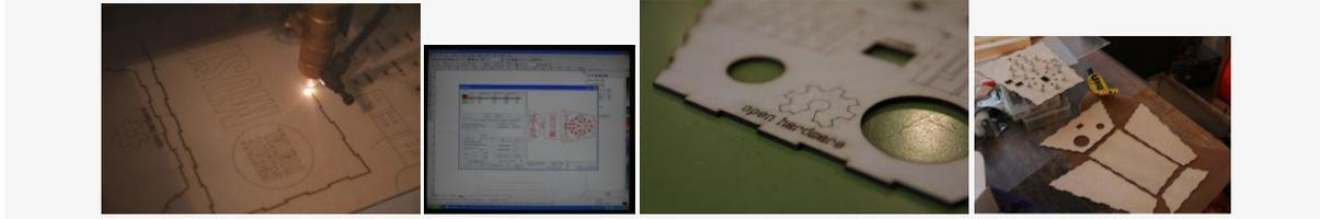
First step is to do the laser-cut enclosure. As I couldn't find any laser-cutting facilities with a powerful machine, I didn't have much choice in wood; it had to be 2mm or thinner. Most types of wood are quite weak and flexible at that thickness, so I had quite a search finding the right wood. I finally settled to a beech plywood for model airplanes of 'F1' quality, whatever that means.
