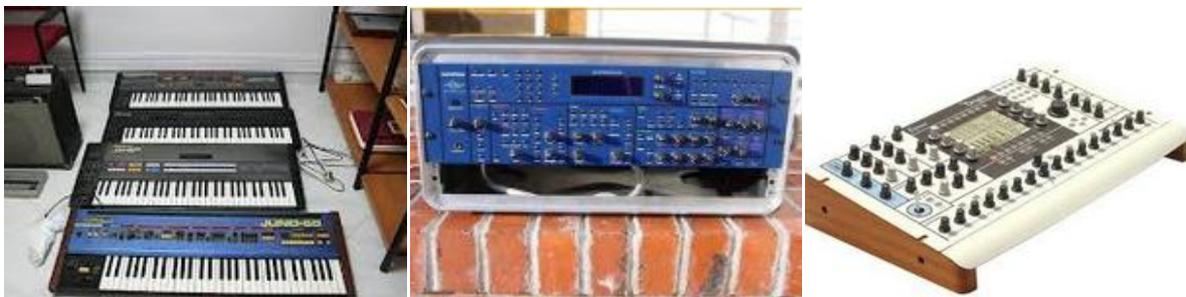
FIGURE 7. THREE COMMON FORM FACTORS FOR SYNTHESIZERS (KEYBOARD, RACK-UNIT, TABLETOP)
