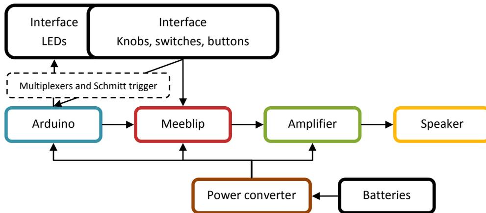
FIGURE 37. DIAGRAM OF ELECTRONIC STRUCTURE
