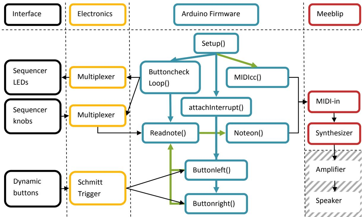
FIGURE 44. DIAGRAM OF THE ELECTRONICS AND FIRMWARE ARCHITECTURE
