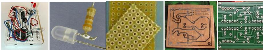
FIGURE 38. BREADBOARD, WIRE-TO-WIRE, PROTOBOARD, DIY PCB, PCB
