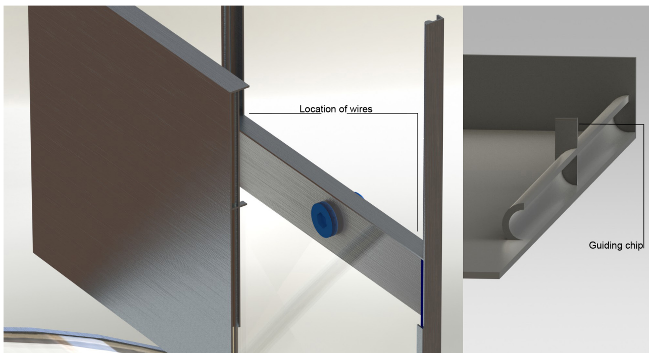
Fig 7.09: Covering plate and click system.
